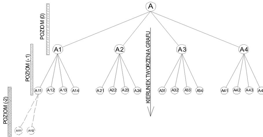
Fig. 5. The graph of dimensional chains hierarchy
