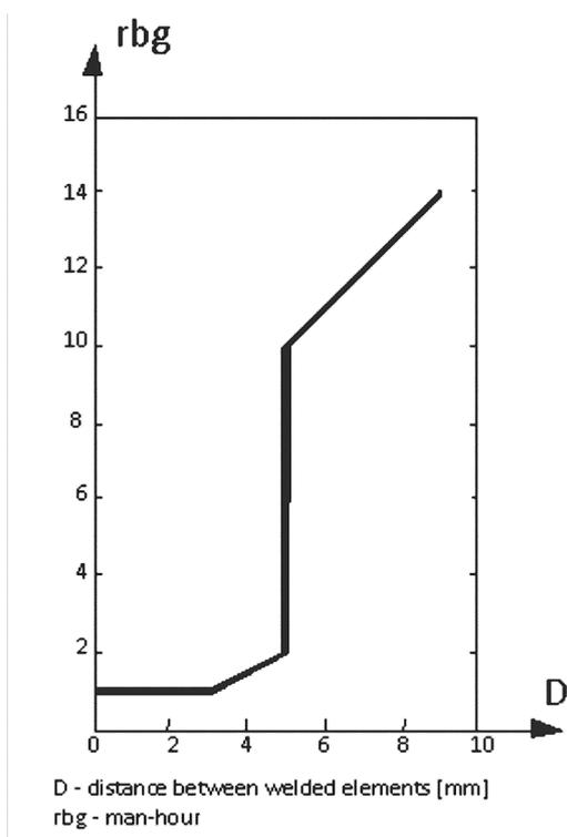
Fig. 4. Relationship between the workload of welding and distance between welded elements [2]
