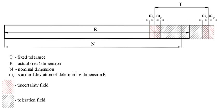
**Fig. 3.** Position of dimension in relative to nominal dimension
