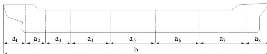
Fig. 2. The basic dimensional chain of a ship’s hull
