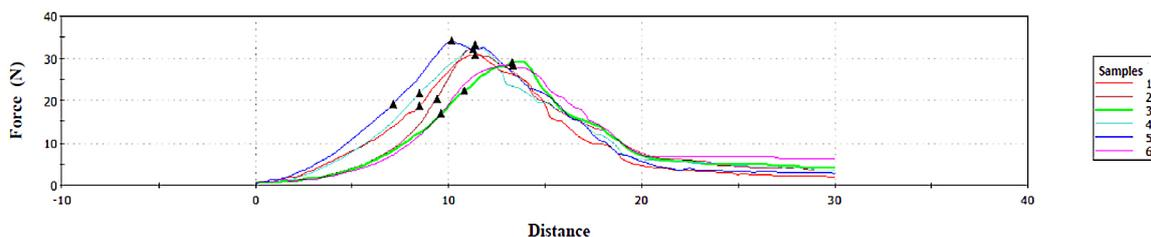
Fig. 2. Example of graph of instrumental texture measurement
