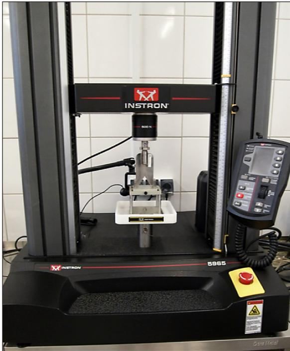
Fig. 1. Texture analysis equipment with the V-blade
