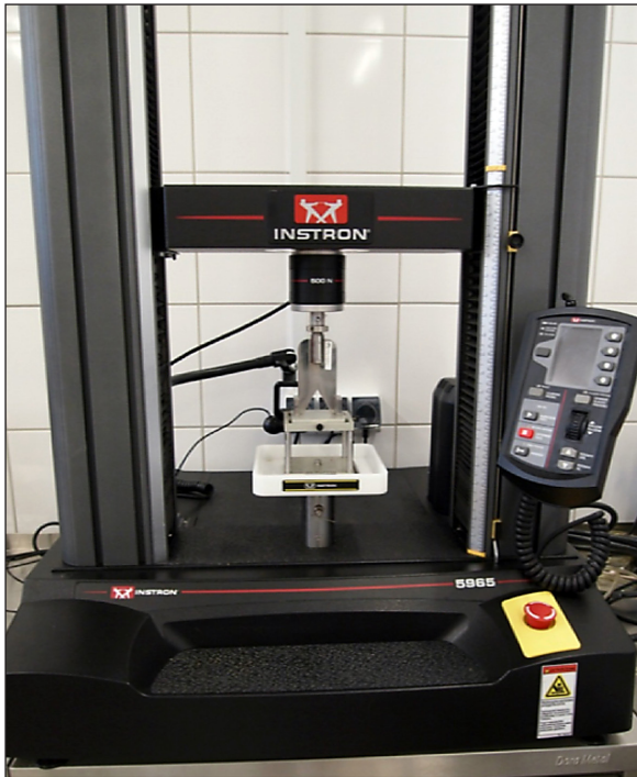
Fig. 1. Texture analysis equipment with the V-blade
