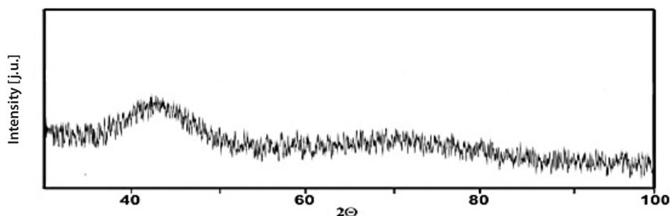
**Fig. 2.** The X-ray diffraction patterns obtained for amorphous alloy strip  $\text{Co}_{22}\text{Y}_{54}\text{Al}_{24}$
