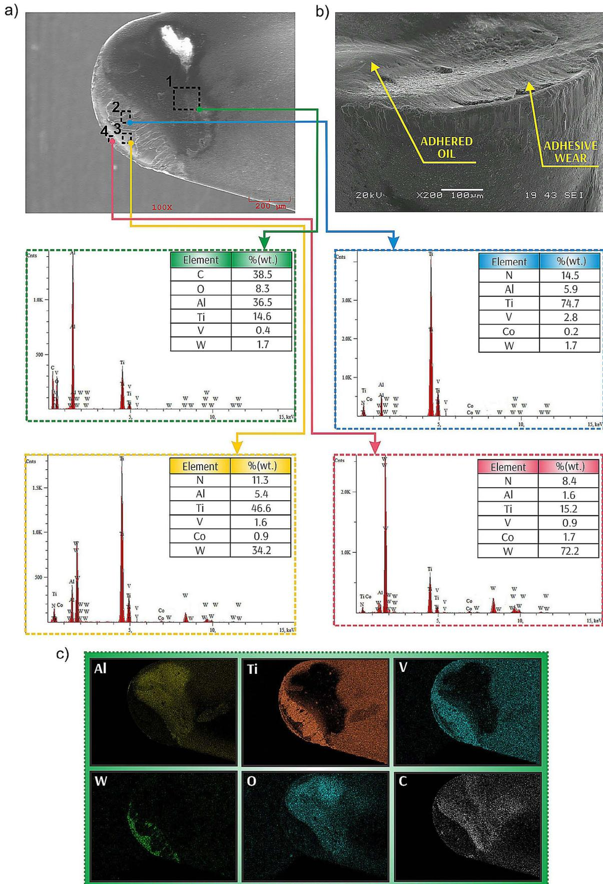
**Figure 7.** SEM of cutting tool with 1 wt% Al<sub>2</sub>O<sub>3</sub> nanoparticles at (a) Rake face (b) Flank face and (c) EDS mapping of cutting tool
