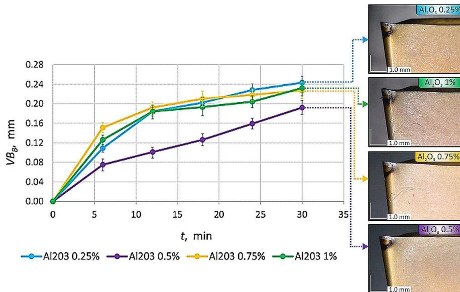
**Figure 2.** Flank wear results with respect to the different ratio of Al<sub>2</sub>O<sub>3</sub> nanoparticles
