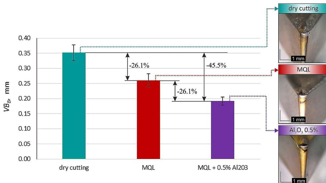
Figure 8. Flank wear results under different cooling conditions
