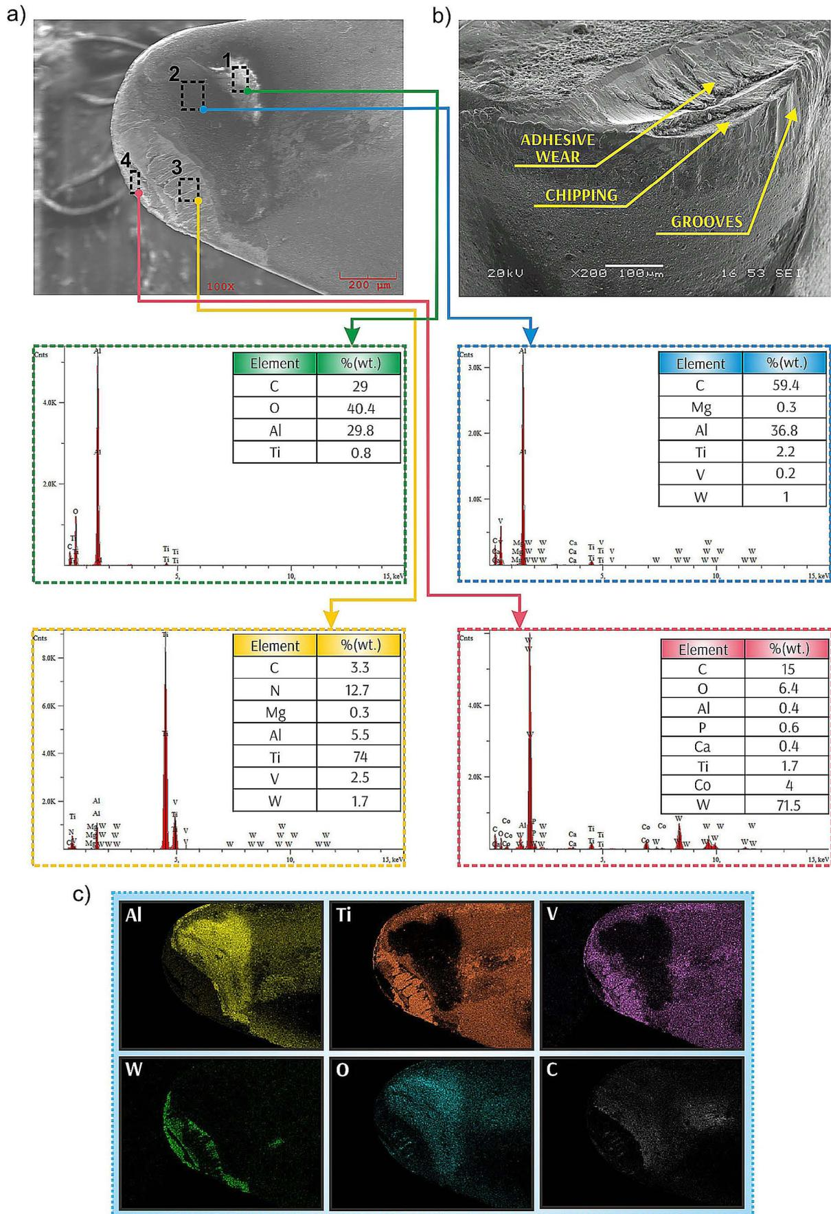
**Figure 4.** SEM of cutting tool with 0.25 wt%  $\text{Al}_2\text{O}_3$  nanoparticles at (a) Rake face (b) Flank face and (c) EDS mapping of cutting tool
