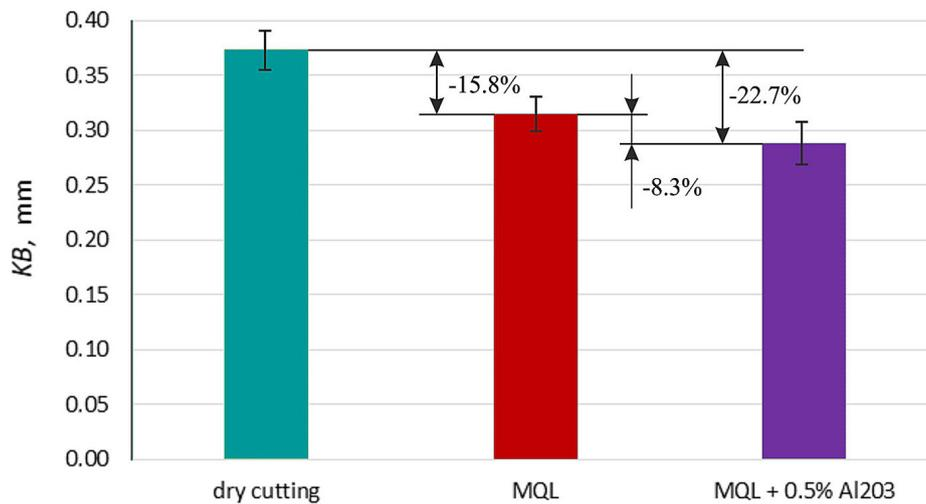
**Figure 9.** Crater wear results under different cooling conditions
