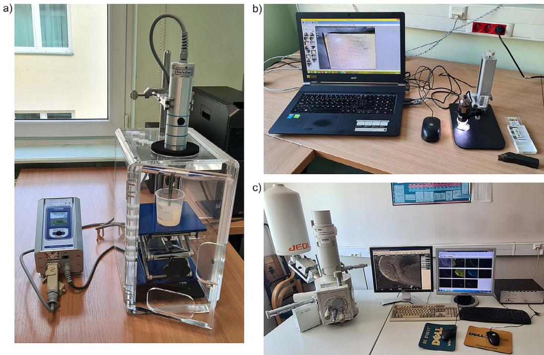
**Figure 1.** Apparatus used for the research: (a) Hielscher UP200St ultrasonic homogenizer, (b) Dino Lite AM7013MZT digital microscope, (c) JEOL JSM-5600LV SEM microscope
