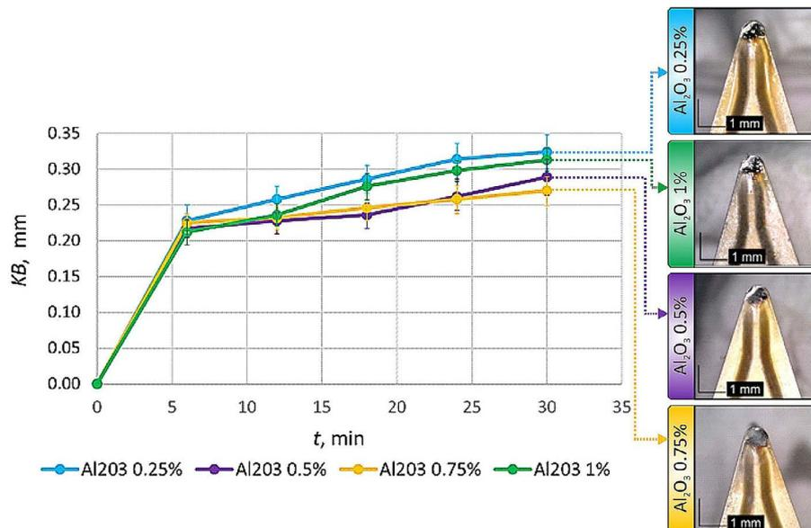
**Figure 3.** Crater wear results with respect to the different ratio of  $\text{Al}_2\text{O}_3$  nanoparticles
