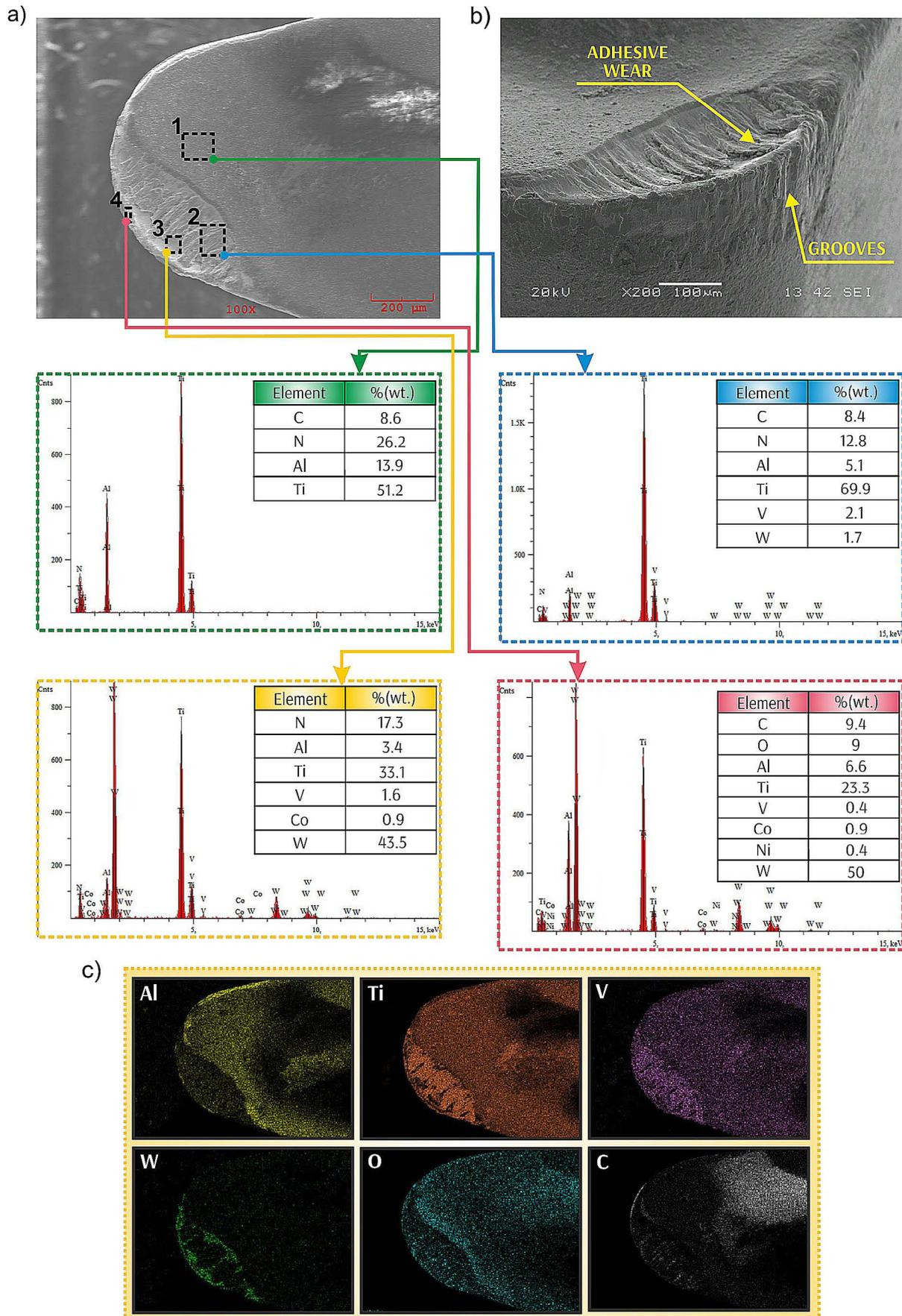
**Figure 6.** SEM of cutting tool with 0.75 wt% Al<sub>2</sub>O<sub>3</sub> nanoparticles at a) Rake face (b) Flank face and (c) EDS mapping of cutting tool
