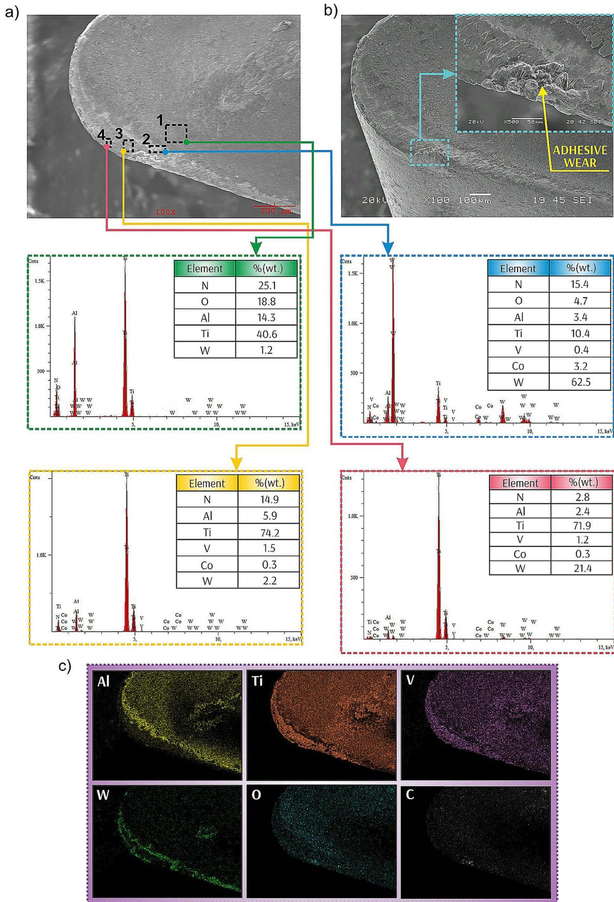
**Figure 5.** SEM of cutting tool with 0.5 wt% Al<sub>2</sub>O<sub>3</sub> nanoparticles at (a) Rake face (b) Flank face and (c) EDS mapping of cutting tool
