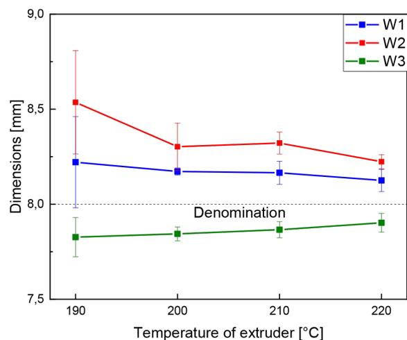
**Figure 1.** Correlation of nozzle temperatures and rollers deformation
