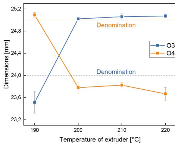
**Figure 3.** Correlation of nozzle temperatures and designated distances
