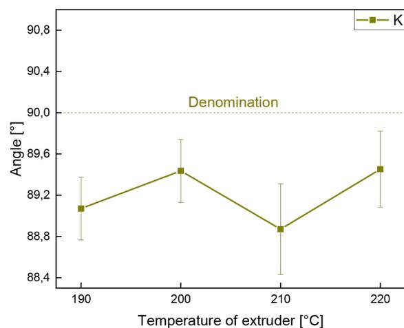
**Figure 2.** Correlation of the nozzle temperatures and the angle between the cylinder and plane
