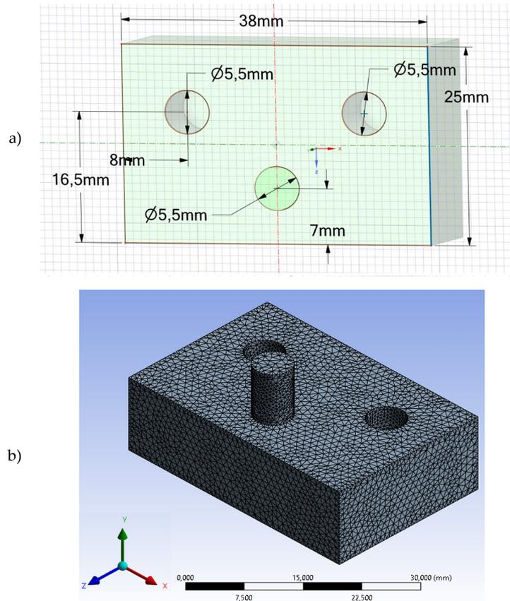
Figure 5. Model of the tested sample: a) dimensions of PLA 3D model solid with different printing temperatures; b) mesh of the PLA solid
