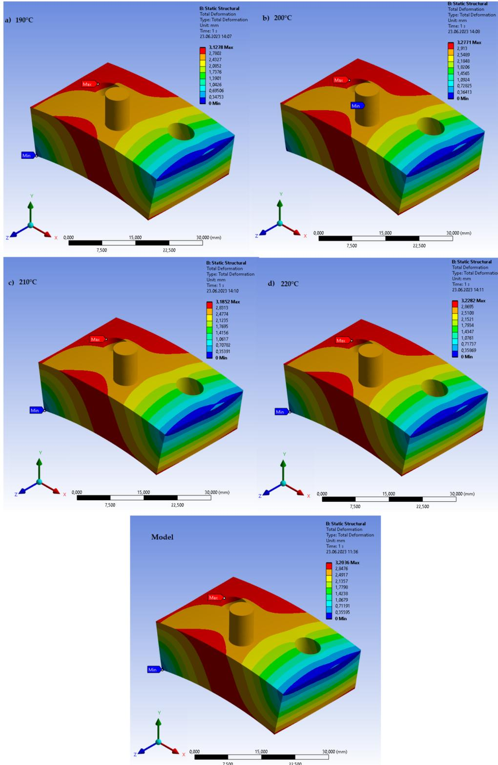
Figure 11. FEM analysis of deformations occurring in the designed solid for four nozzle temperatures and reference model during bending
