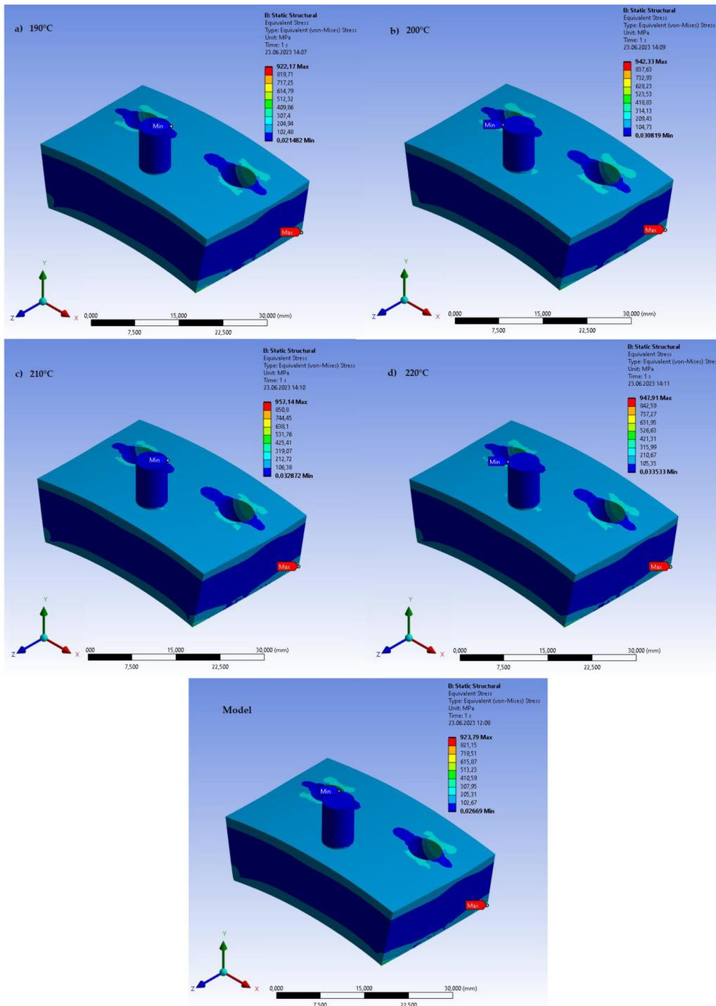
Figure 10. FEM analysis of stresses occurring in the designed solid for four temperatures of the nozzle and reference model during bending
