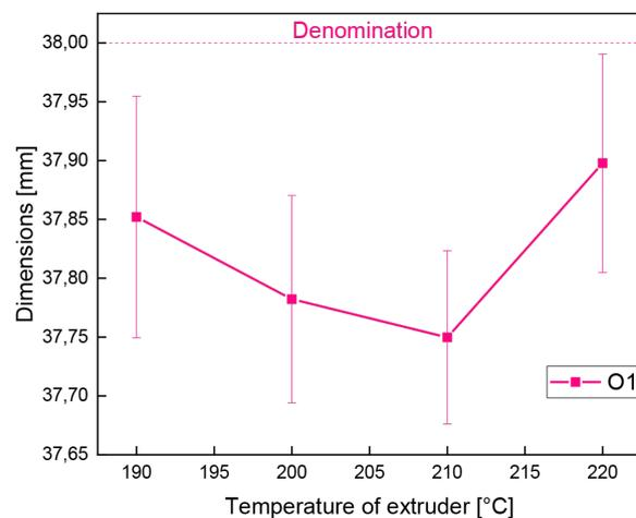
**Figure 4.** Correlation of nozzle temperatures and the distance between the centers of the rollers W1 and W2
