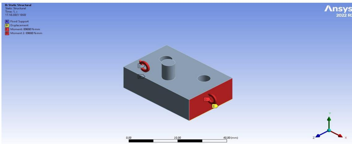
Figure 7. Scheme of performed one-point bending with fixed force
