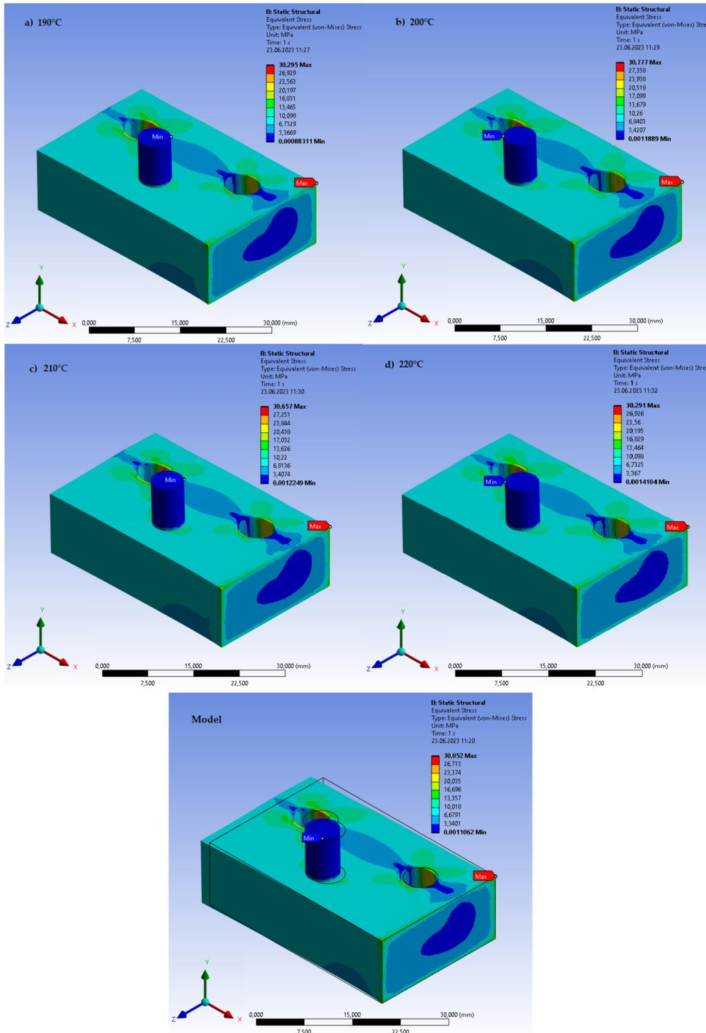
Figure 8. FEM analysis of stresses occurring in the designed solid for four temperatures of the nozzle and reference model during stretching
