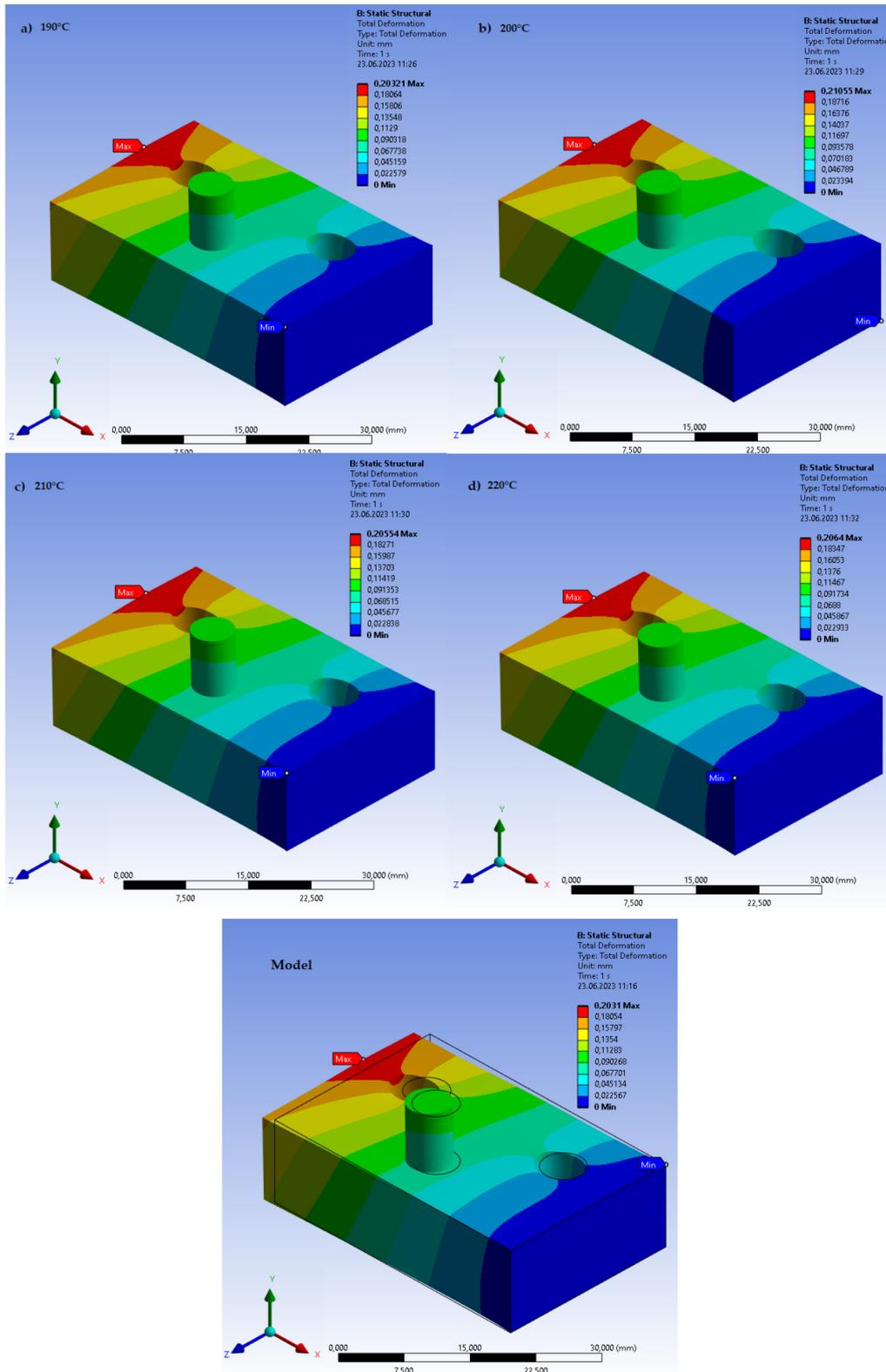
Figure 9. FEM analysis of deformations occurring in the designed solid for four temperatures of the nozzle and reference model during stretching
