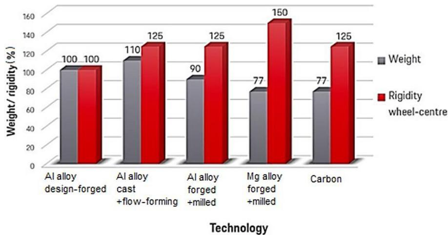
Fig. 1. Weight/rigidity comparison of certain wheel materials and technologies [2]
