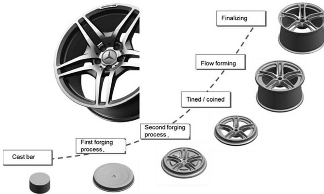
Fig. 2. Forging process [11]
