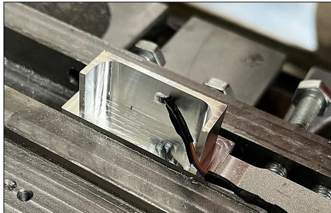
Fig. 6. Location of the resistance temperature sensor on the sample
