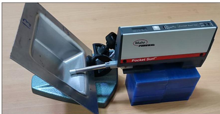
**Fig. 7.** The measurement process of the surface roughness
