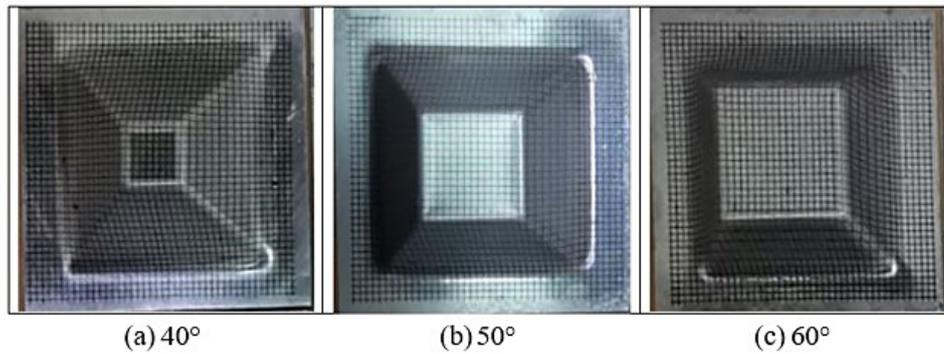
**Fig. 6.** The products produced using the SPIF process for the wall angles: (a) 40°, (b) 50° and (c) 60°
