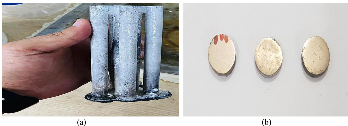
Fig. 1. Photo of specimen (a) the ingot, (b) after cutting
