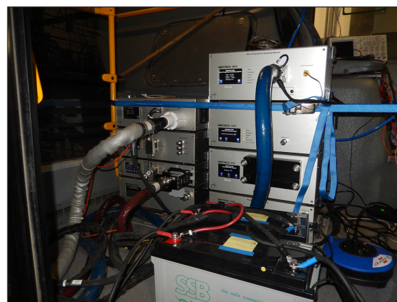
Fig. 3. Exhaust gas analyser fitted to the test vehicle
