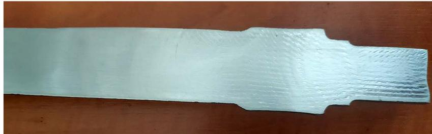
Fig. 16. Axial section of a rolled axle
