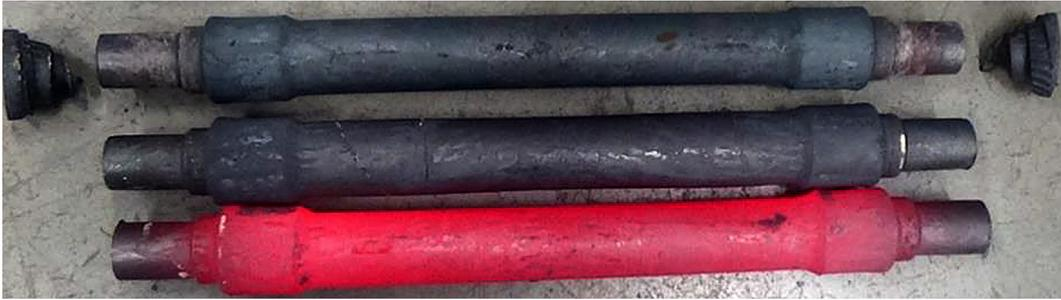
Fig. 15. Railcar axles rolled in 1:6 scale at the Lublin University of Technology
