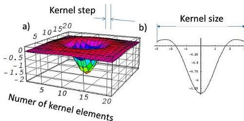
Fig. 12. Laplacian of Gaussian function: (a) 2D kernel of the LoG, (b) 1D kernel LoG
