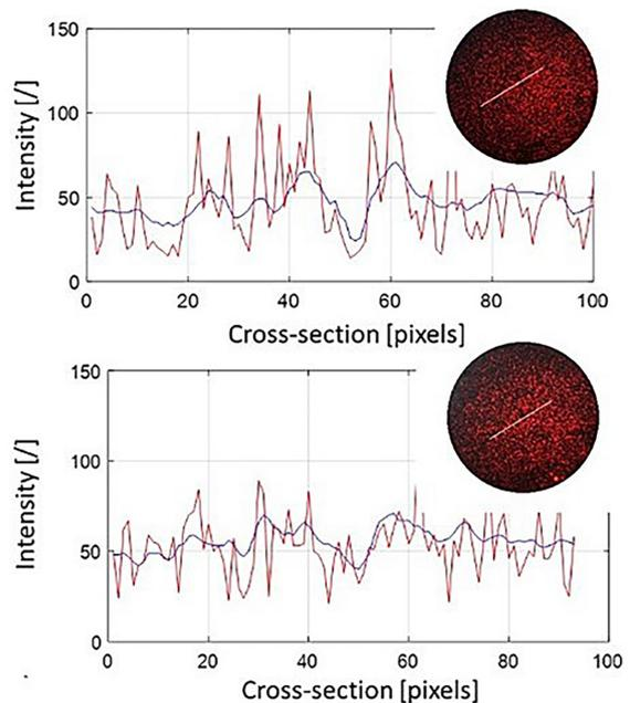
Fig. 15. Courses of the crack cross-section for two smaller magnifications with Gaussian smoothing
