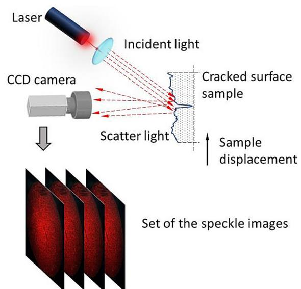
Fig. 5. Schematic of the concept for the laser speckle investigation
