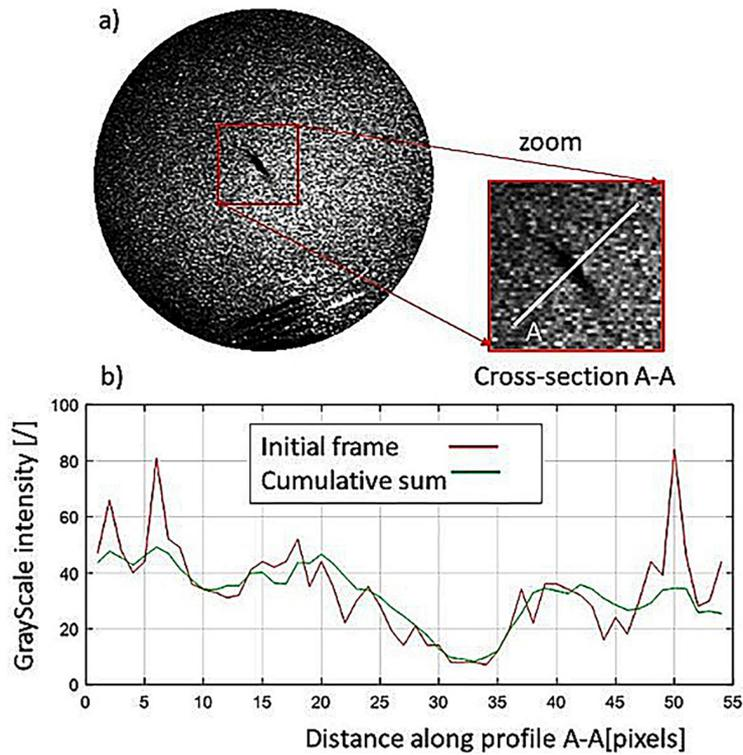
Fig. 7. Shifting-and-add results: a) cumulative sum, b) intensity of the line section for first image (red line), cumulative images (blue line)
