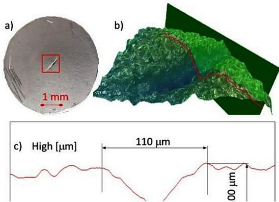
**Fig. 3.** Sheet metal crack characteristics: (a) surface crack, (b) 3D crack identification, (c) crack measurement profile
