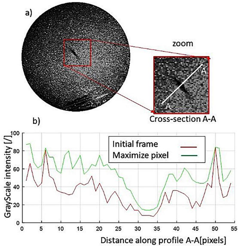
Fig. 8. Shifting-and-add results: (a) maximized pixels, (b) intensity of the line section for first image (red line), cumulative images (blue line)
