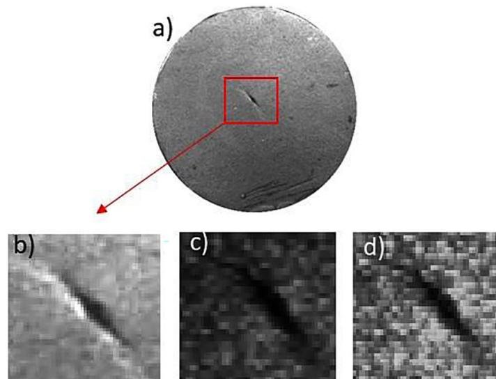
**Fig. 10.** (a) Image under regular lighting (reference image – white light), (b) selected crack for reference image, (c) selected crack for averaging algorithm, (d) select crack for maximized pixel algorithm
