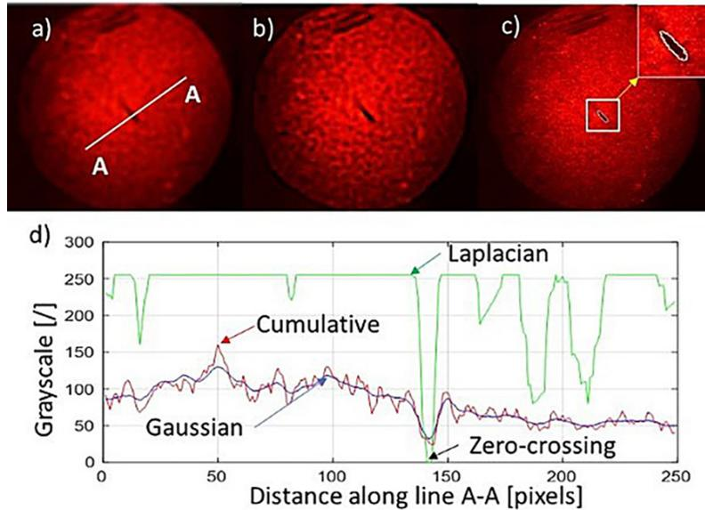
Fig. 13. Results of the digital image processing: a) lower-pass filter (smoothing), (b) high-pass filter (Laplacian), (c) zero crossing edge detection
