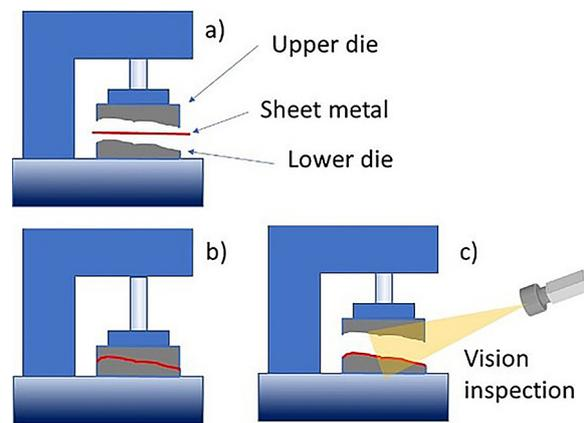
Fig. 1. Sheet metal forming; (a) forming components, (b) the concept of the sheet metal forming inspection
