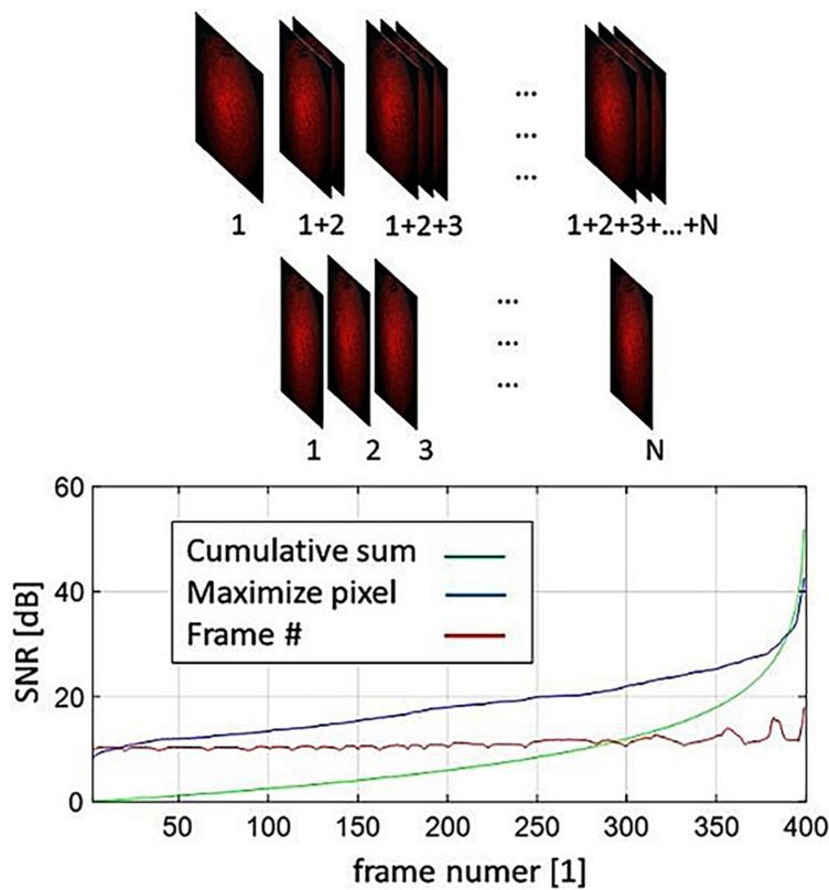
Fig. 9. Signal-to-noise evaluation for the maximized pixels (blue line), average (green line) and original images (red)
