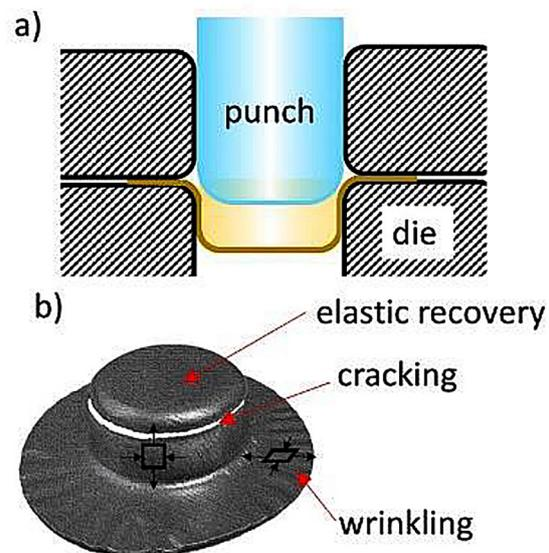
Fig. 2. Typical sheet metal defects: (a) schematic drawing, (b) cracking and wrinkling (own elaboration)
