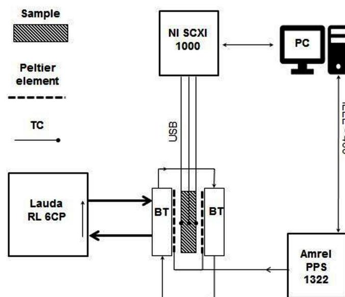
Fig. 2. Scheme of the test stand for thermal diffusivity tests using the modified Ångström method. Head in a configuration for bilateral forcing tests, BT - thermostatic blocks
