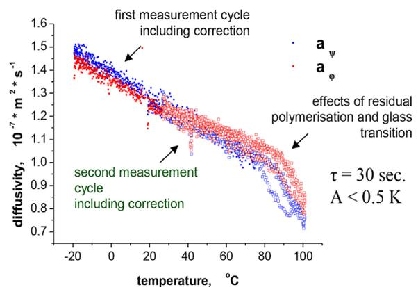
**Fig. 6.** Comparison of the results of the first and second thermal diffusivity tests for a resin sample with 0% nano-dispersion filling
