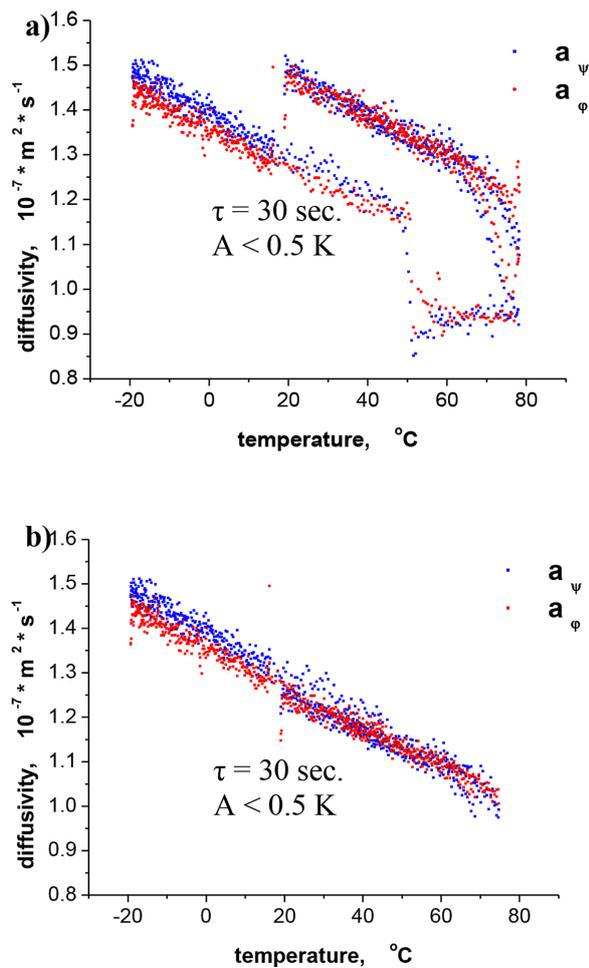
**Fig. 5.** Results of thermal diffusivity tests from the first measurement cycle for a resin sample with 0% nano-dispersion filling before (a), and after (b) dilatation correction
