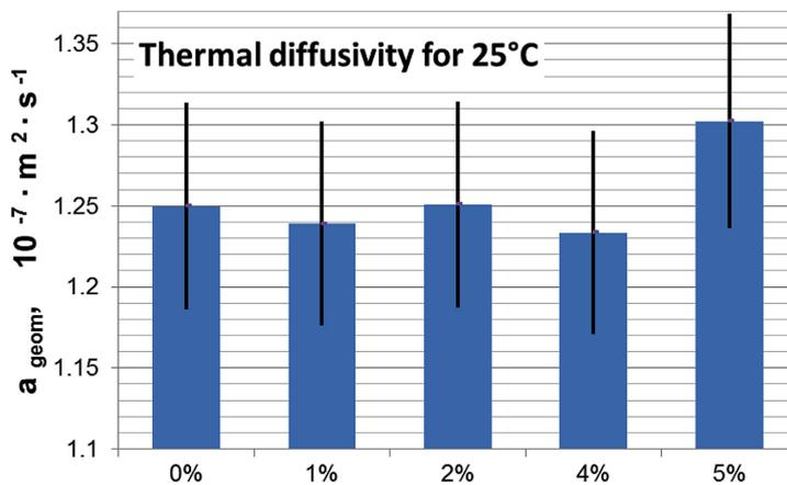
Fig. 8. Comparison of the geometric mean value of the thermal diffusivity at 25  $^{\circ}C$  of the entire range of 0% to 5% nano-dispersion additives
