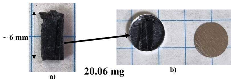
Fig. 4. DSC test sample in the initial state (a) and placed to the sample pan (b; sample pan lid on the right)
