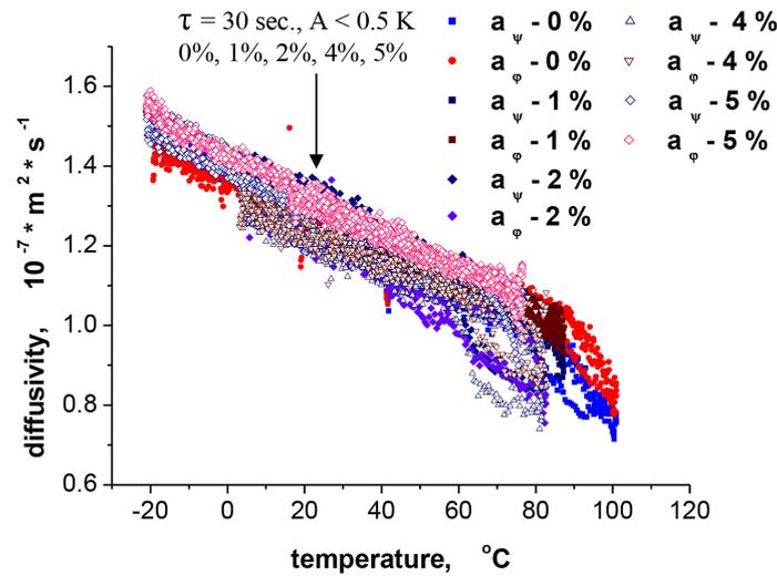
Fig. 7. Comparison of thermal diffusivity test results for the entire range of samples from 0% to 5% nano-dispersion addition
