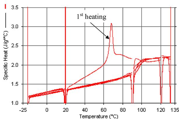
**Fig. 9.** Temperature characteristics of the specific heat of the resin (LH145H147) obtained for 1 and 2 heating/cooling cycles
