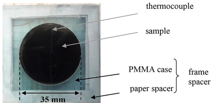
Fig. 3. Test specimen in bilateral forcing configuration
