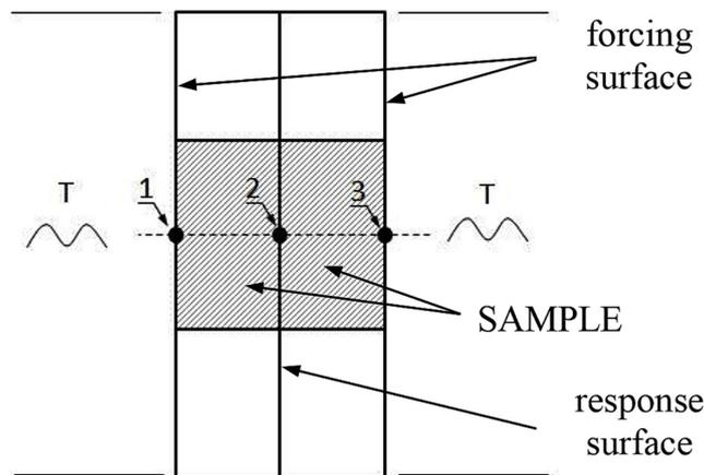
Fig. 1. Diagram of bilateral thermal forcing (b), 1,3 – readout points of the forcing signal, 2 – readout points of the response signal
