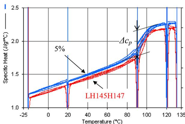
**Fig. 10.** Temperature characteristics of the specific heat of the resin (LH145H147) and the composite structure with 5% volume of nanotubes (5%) obtained for the heat-stabilized state – 1 cooling and 2 heatings and coolings
