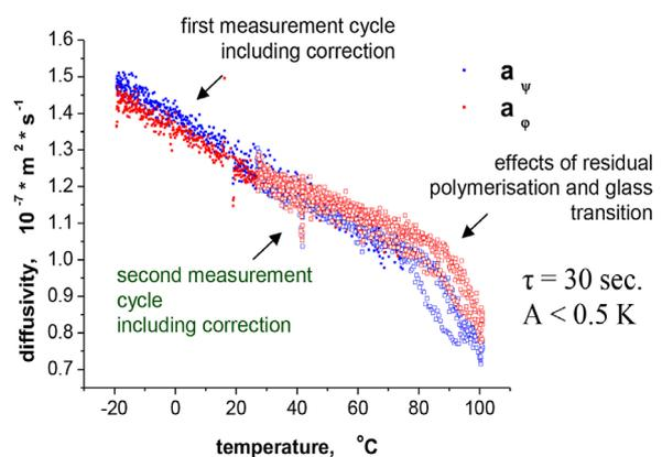
Fig. 6. Comparison of the results of the first and second thermal diffusivity tests for a resin sample with 0% nano-dispersion filling
