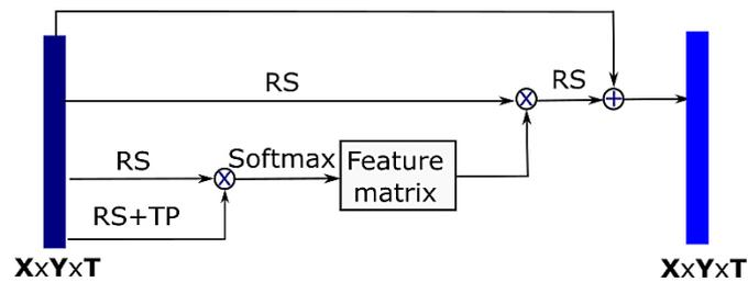
Fig. 2. General scheme of attention module. RS represents matrix reshaping, TP matrix transposition
