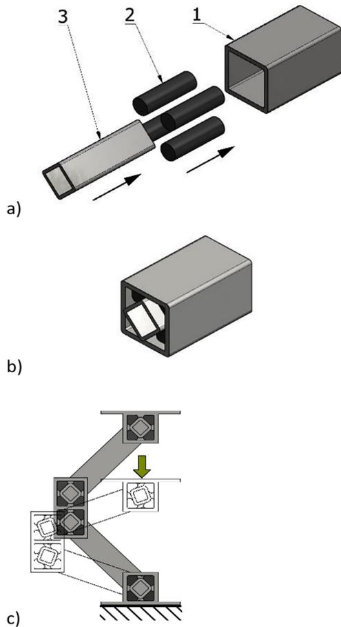
**Fig. 4.** Design of the Neidhart spring; a) disassembled spring, 1 – square shaft, 2 – cylindrical elastomer inserts, 3 – main body; b) assembled spring; c) four-joint elastic mount
