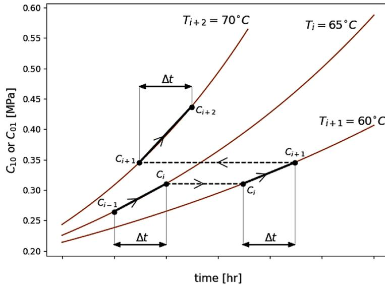
Fig. 7. Method of calculating new values of  $C_{10}$  and  $C_{01}$  parameters for consecutive time periods based on Arrhenius equations and selected temperatures
