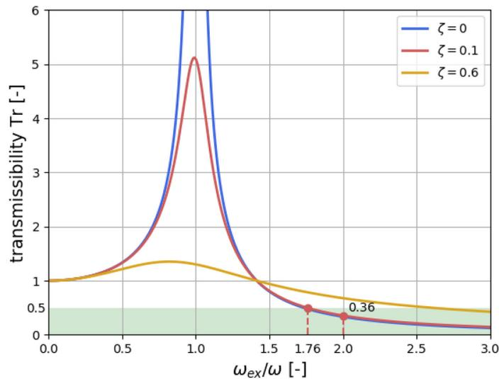
Fig. 1. Transmissibility for different damping ratio  $\zeta$  values
