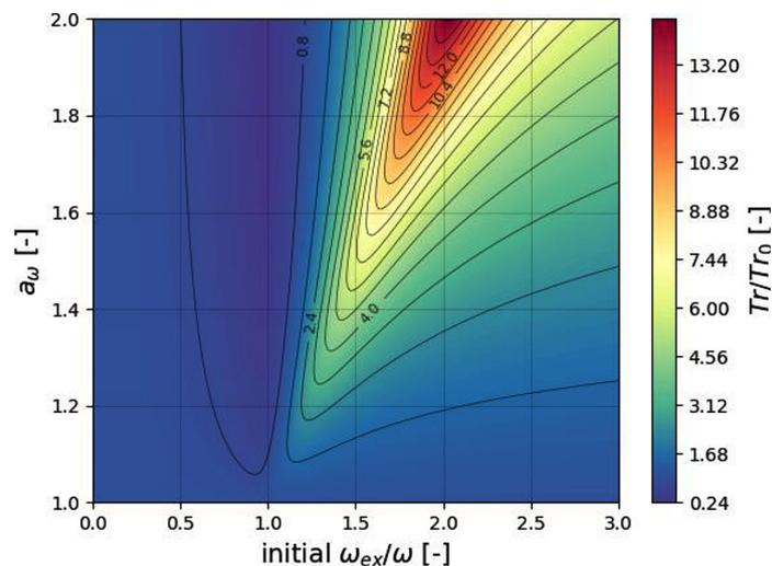
Fig. 2. Relative transmissibility as a function of the initial  $\omega_{ex}/\omega$  and  $a_\omega$  for  $\zeta = 0.1$
