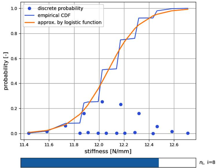
Fig. 10. Example of a partial CDF for a single time period based on a histogram
