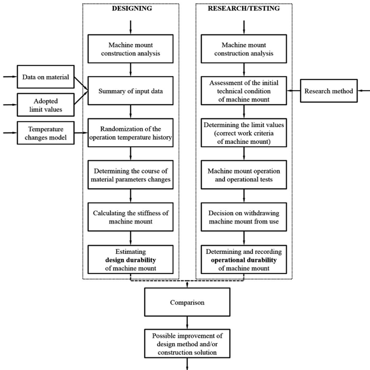
Fig. 5. Diagram of the procedure for estimating the design and operational durability of a machine mount
