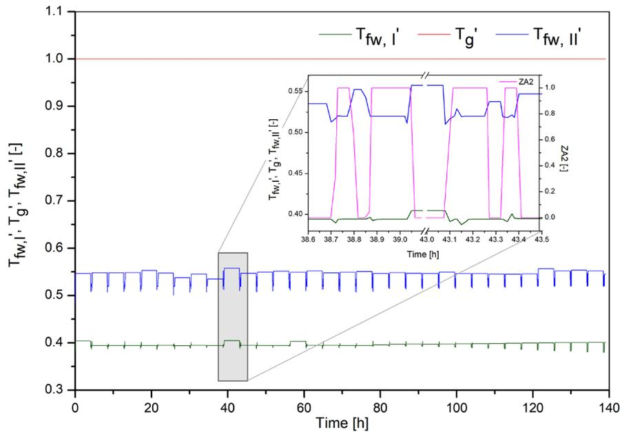
**Figure 9.** The fresh water temperature before ( $T_{fw,I}$ ) and after ( $T_{fw,II}$ ) the HE2 heat exchanger and the glycol temperature ( $T_g$ ) throughout the production cycle and the opening stage of the ZA2 valve
