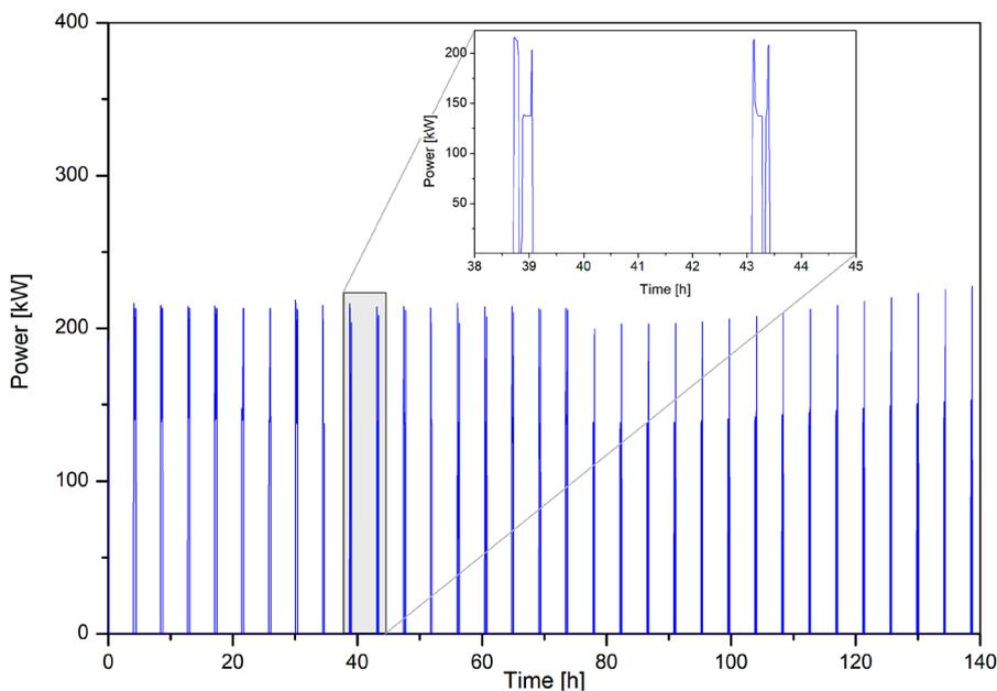
**Figure 10.** Instantaneous power output of the HE2 heat exchanger throughout the production cycle
