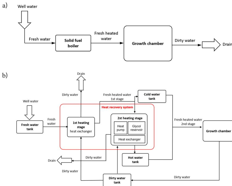
**Figure 1.** Schematic block diagram of a plant for producing vegetable sprouts without (a) and with (b) heat recovery
