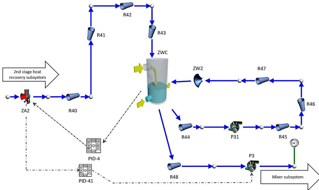
**Figure 6.** Schematic diagram of the model of the hot tank subsystem (ZWC – hot water tank; ZA2, ZW2 – valves; P3, P31 – water pumps; PID-4, PID-41 – PID controllers, R40-R48 - pipelines)
