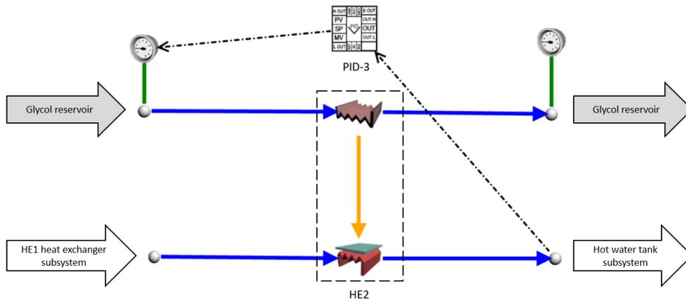
Figure 4. Schematic diagram of the model of the second stage heat recovery subsystem (HE2 – heat exchanger, PID-3 – PID controller)
