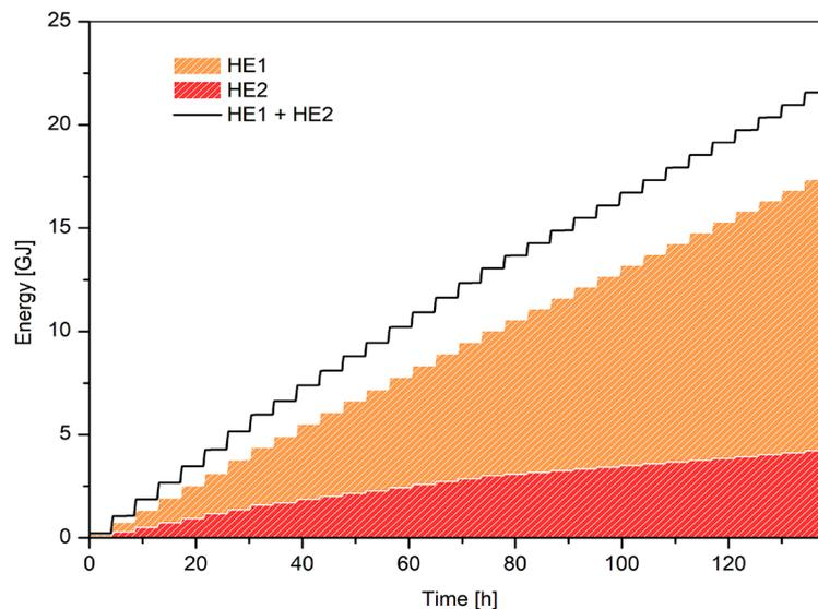
**Figure 11.** Accumulated amount of energy transferred to fresh water in heat exchanger HE1 and HE2
