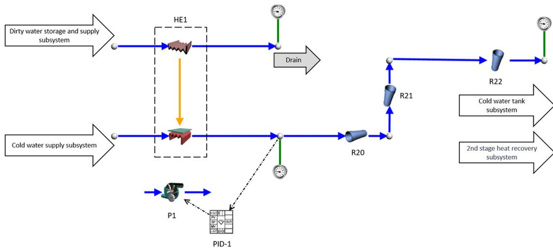
Figure 3. Schematic diagram of the model of the HE1 heat exchanger subsystem (HE1 – heat exchanger, P1 – fresh water pump, R20-R22 - pipelines)
