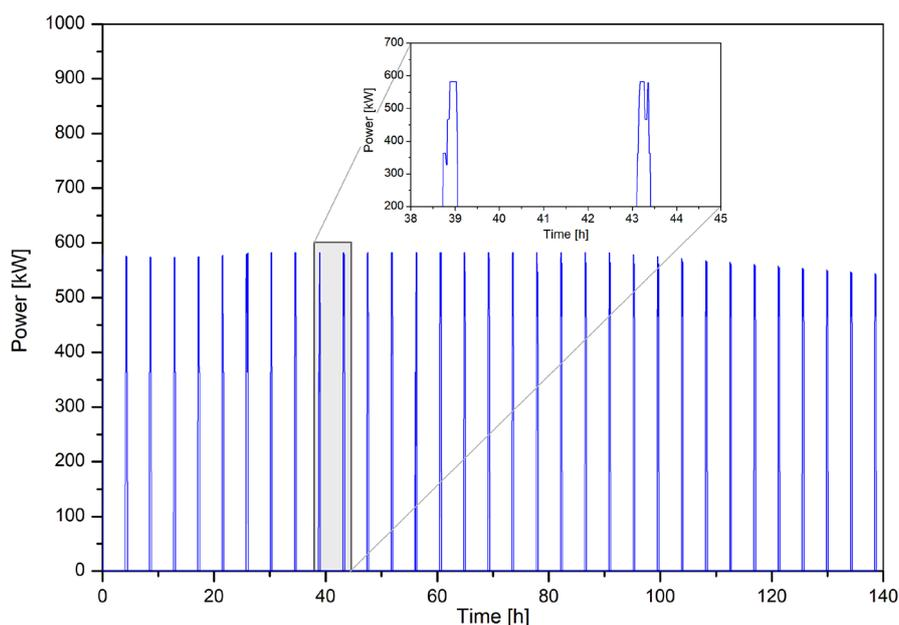
**Figure 8.** Instantaneous power output of the HE1 heat exchanger throughout the production cycle
