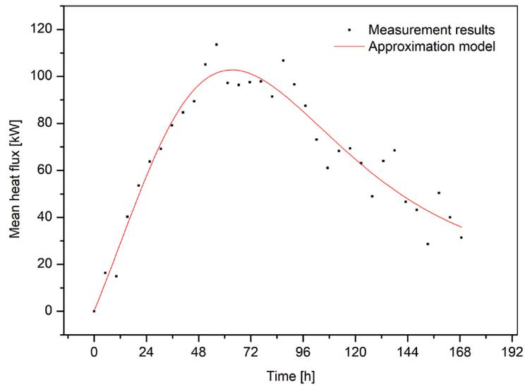
Figure 2. Measurement results for determining the heat generation model by sprouts
