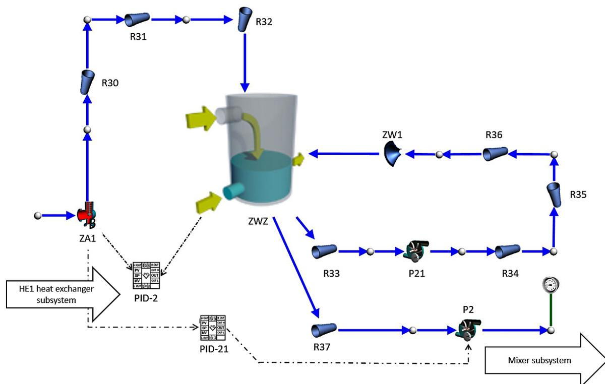
**Figure 5.** Schematic diagram of the model of the cold tank subsystem (ZWZ – cold water tank; ZA1, ZW1 – valves; P2, P21 – water pumps; PID-2, PID-21 – PID controllers, R30-R37 - pipelines)
