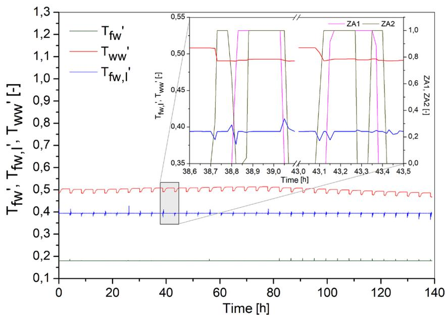
**Figure 7.** The fresh water temperature after ( $T_{fw,l}'$ ) and before ( $T_{fw}'$ ) the HE1 heat exchanger and the dirty water temperature ( $T_{ww}'$ ) throughout the production cycle and the opening stage of the ZA1 and ZA2 valve
