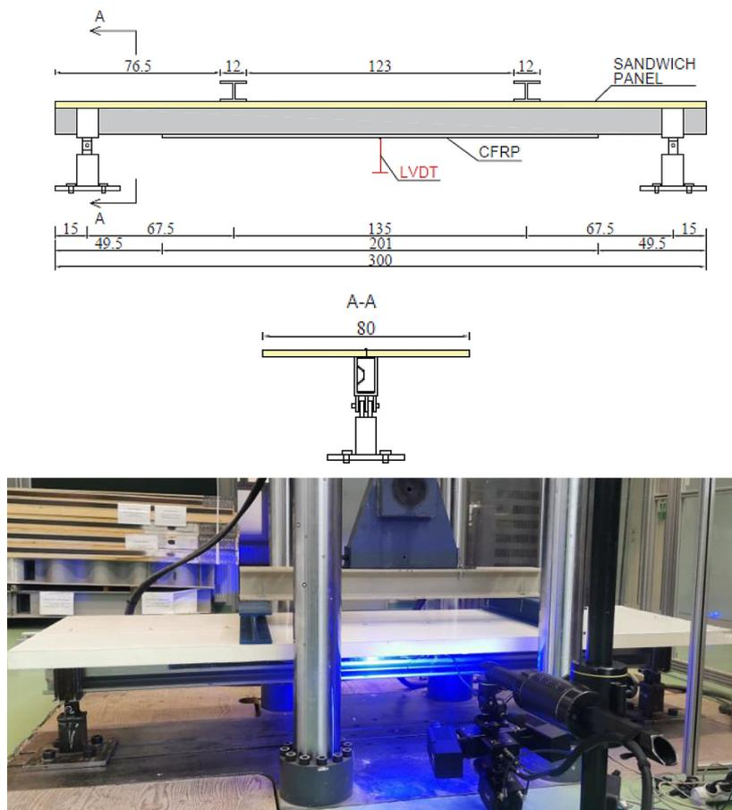
Fig. 3. a) Scheme of the test stand, b) photo of the stand
