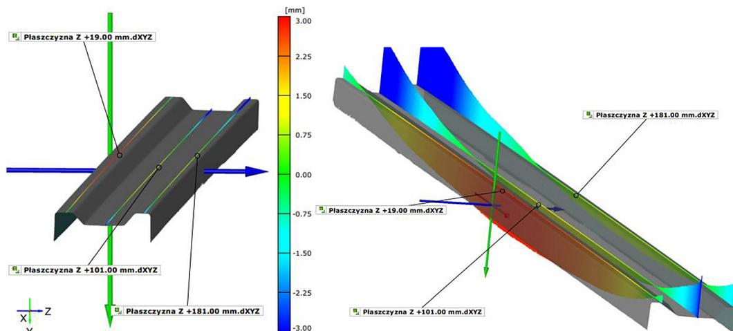
**Fig. 2.** Beam deflection along profile and deflections in relation to CAD model
