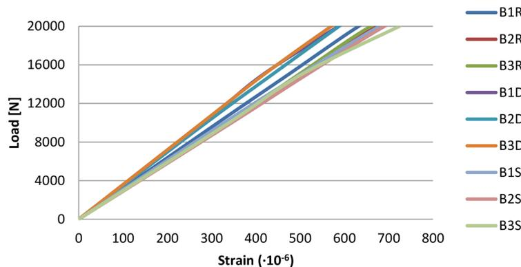
Fig. 6. The graph showing the load-strain relationship at the location of the T2 electro-resistance strain gauge
