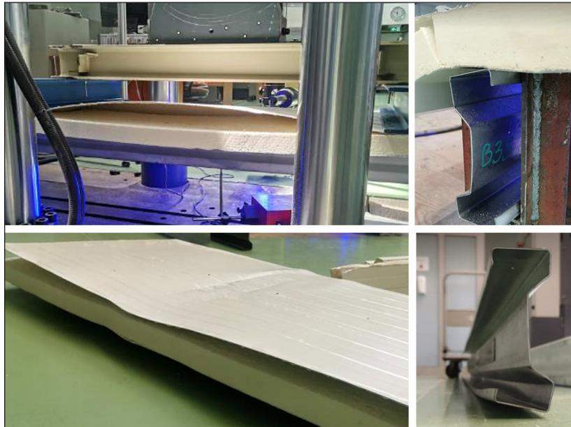
Fig. 4. Typical forms of beam destruction
