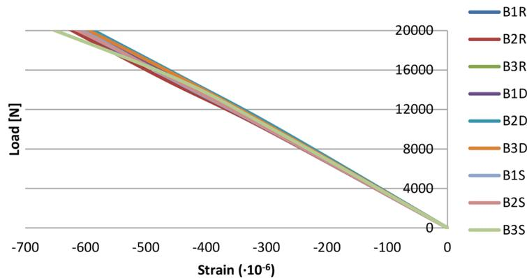
Fig. 5. The graph showing the load-strain relationship at the location of the T1 electro-resistance strain gauge
