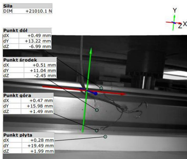
Fig. 8. Presentation of the results of displacement measurements using the Gom Correlate program
