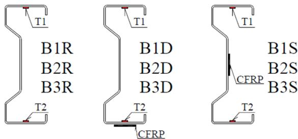
**Fig. 1.** Sample names, location of CFRP tapes and strain gauges T1 and T2
