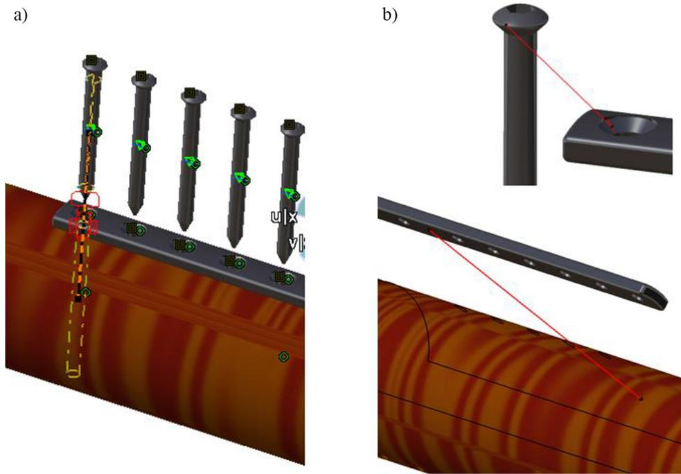
**Figure 3.** Defining connections: (a) Bolt tightening connection, (b) contact connection
