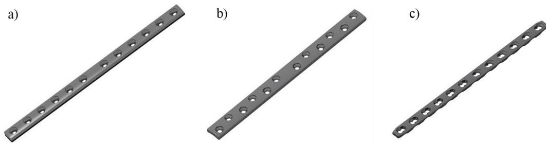
**Figure 1.** The types of analyzed plates, (a) Narrow DCP, (b) Broad DCP, (c) Narrow LCP
