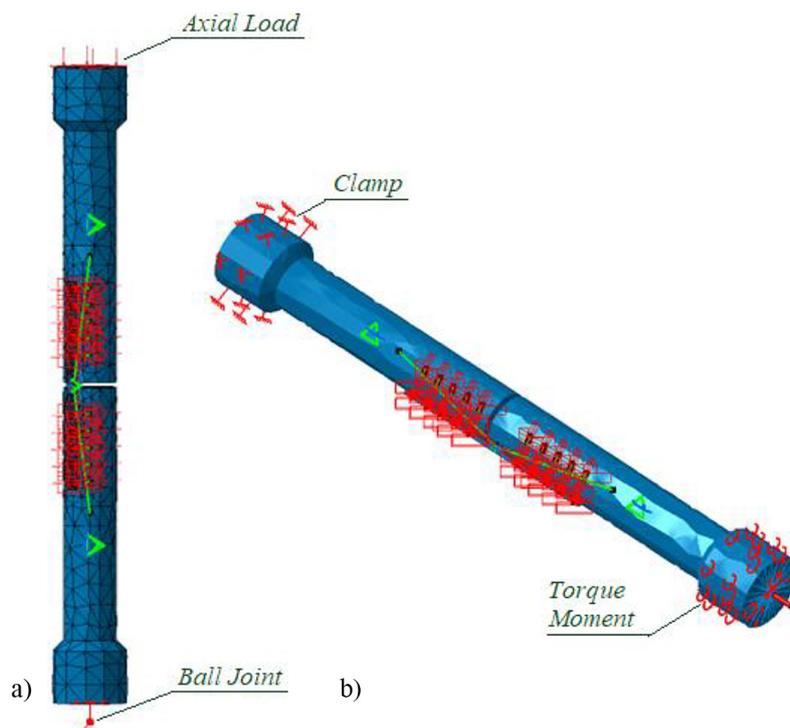
**Figure 4.** Defining constraints and loads: (a) axial load, (b) torque
