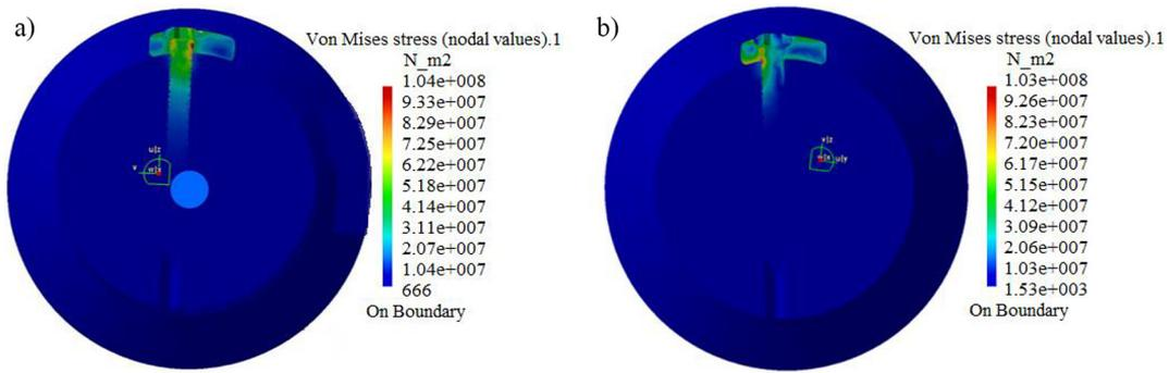
Figure 6. Von Mises stress on the cross-section of the most loaded bolt of a Broad DCP: (a) axial load, (b) torque
