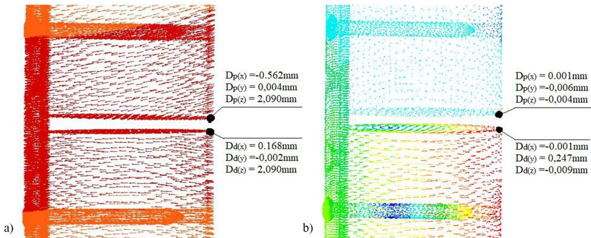
Figure 7. Point displacement vectors for the case of a Broad DCP: a) axial load, b) torque
