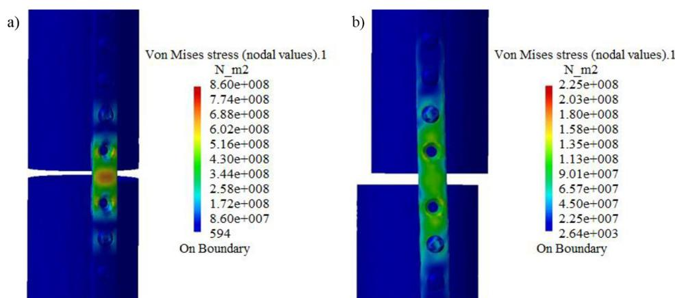
Figure 5. Von Mises stress on a Narrow LC-DCP: (a) axial load, (b) torque
