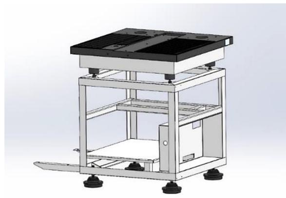
Fig. 6. Frame unit with dampers
