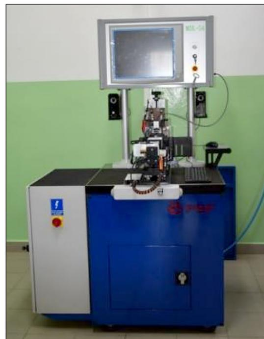
Fig. 1. MDL-54 device for measurements of ball bearing vibration levels
