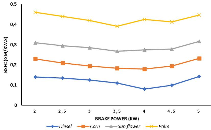
Figure 4. Break-specific fuel consumption vs brake power
