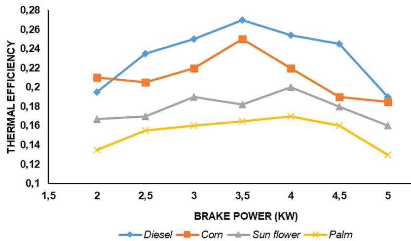
Figure 6. Thermal efficiency vs brake power
