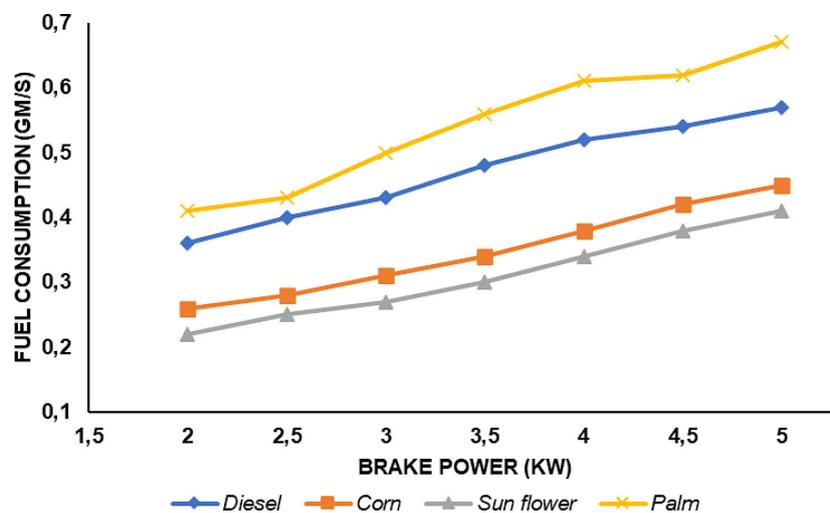
Figure 3. Fuel consumption vs brake power
