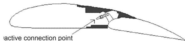
Fig. 6. Schematic of the wing flaps [7]
