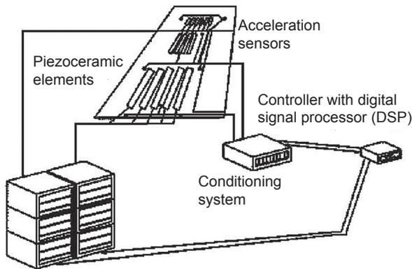
Fig. 4. Vibration Reduction Scheme of the tail of the aircraft
