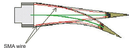
Fig. 7. Schematic of layout of wires comprising a shape memory material [7]
