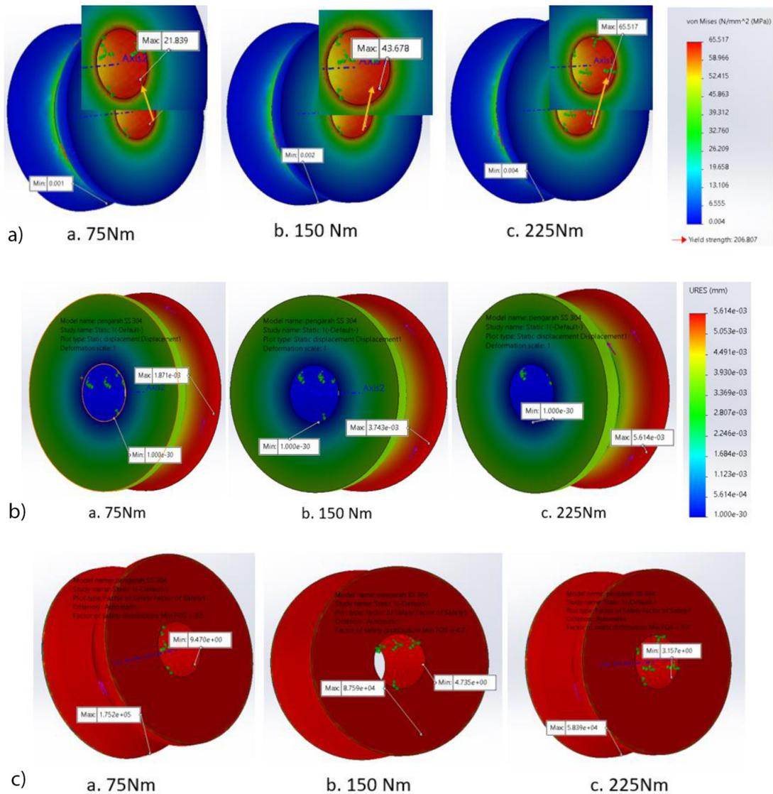
**Fig 7.** The result of the FEA simulation on the additional pulley using Solidworks software, (a) von mises stress, (b) the displacement occurs, (c) factor of safety
