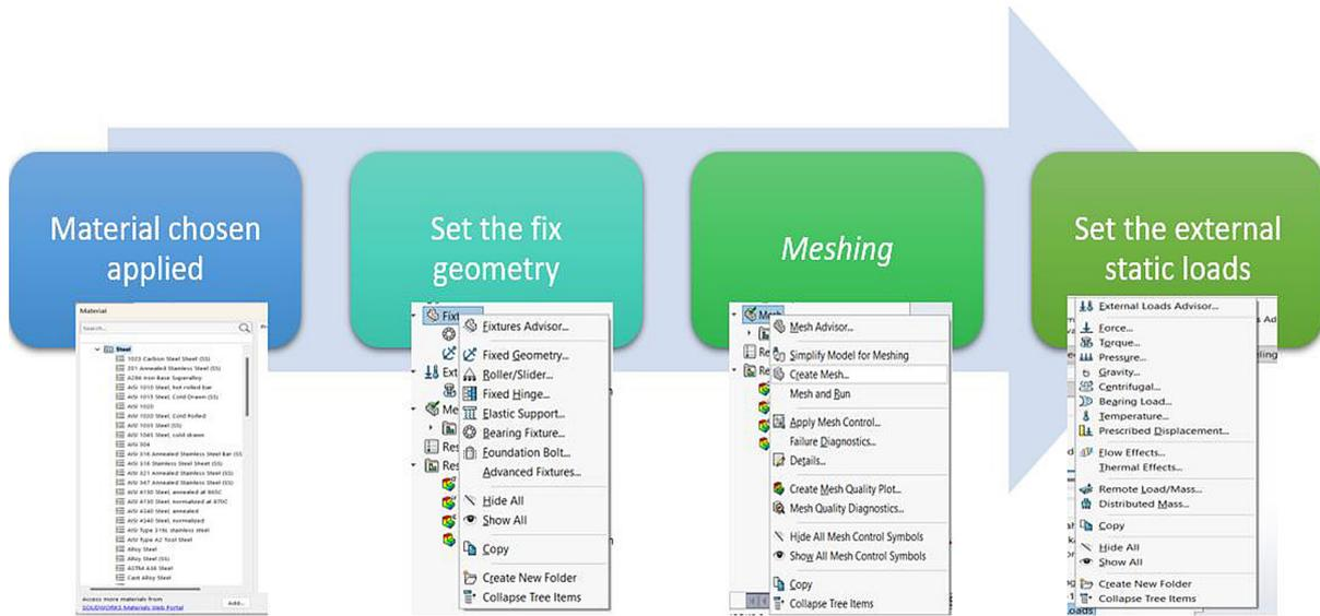
Fig 2. Steps of FEA using Solidworks Software
