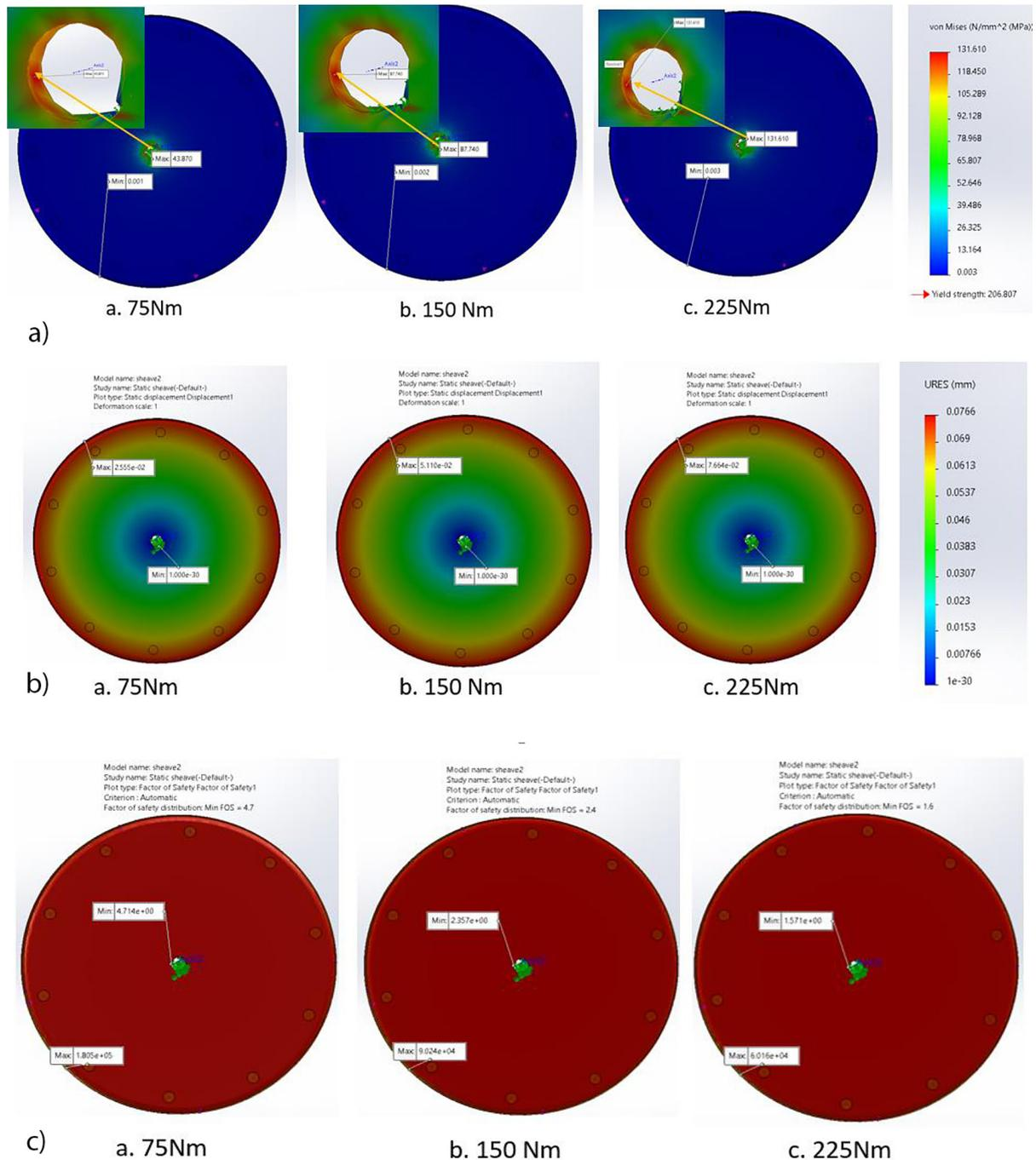
**Fig 5.** The result of the FEA simulation on the line spool plate using Solidworks software, (a) von mises stress, (b) the displacement occurs, (c) factor of safety
