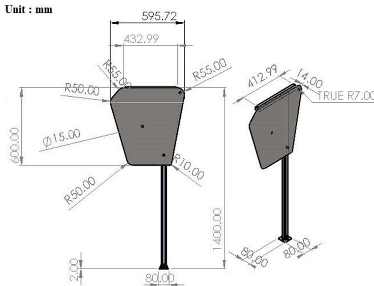
Fig 3. The geometry drawing of Pot hauler and the overall dimension
