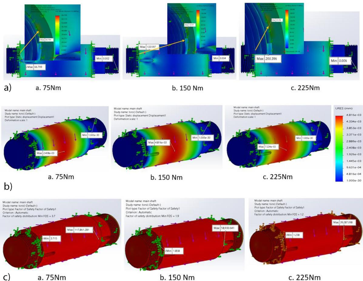
Fig 6. The result of the FEA simulation on the line spool plate shaft's using Solidworks software, (a) von mises stress, (b) the displacement occurs, (c) factor of safety
