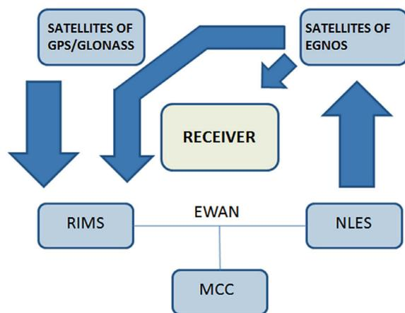
Fig. 2. Principle of operation of EGNOS system
