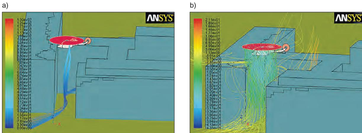
**Fig. 4.** Disturbances caused by helicopter during roof helipad operations:
