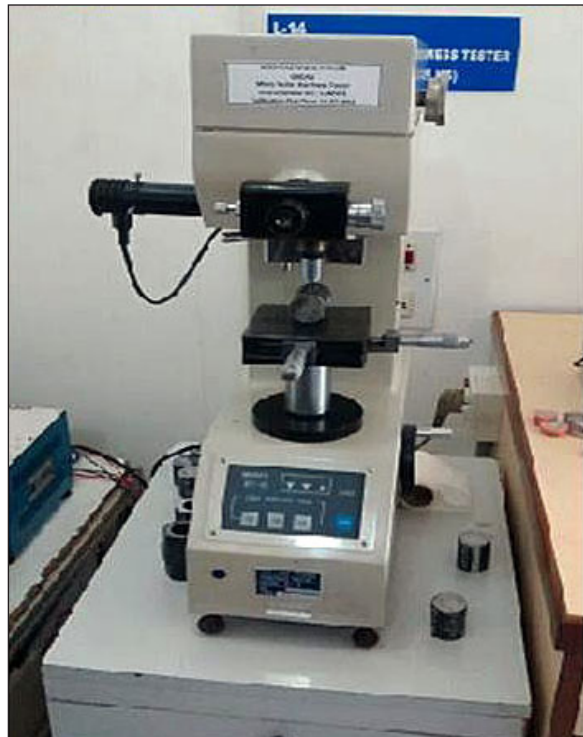
Figure 1. Vickers hardness tester
