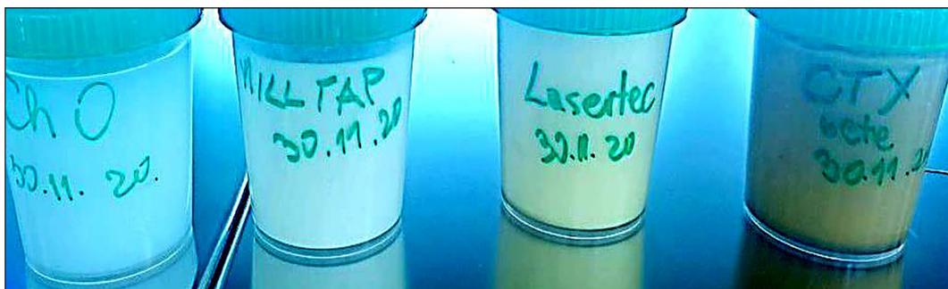
Fig. 2. Samples of pure coolant (a) not used in machining (Ch0) and used respectively from the tanks of the following machines: (b) four-axis milling machining center MILLTAP 700, (c) five-axis milling machine LASERTEC 65 SAUER, d) numerically controlled lathe CTX beta 1250 TC
