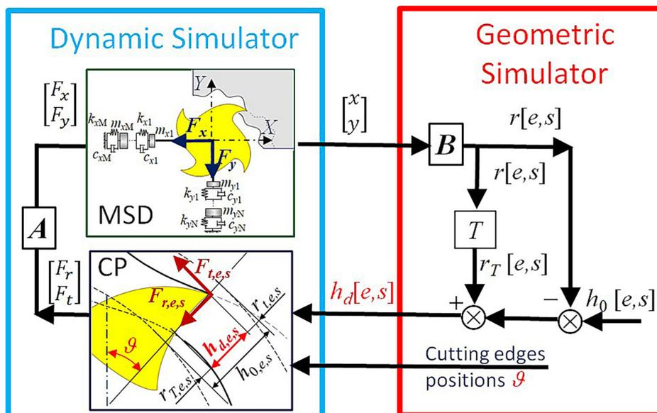
Figure 5. Dynamic machine-tool-workpiece – cutting process system
