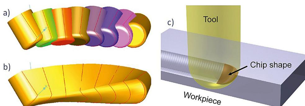
**Figure 1.** Discretization of the tool movement: (a) tool at different NC positions, (b) approximated sweep surface, (c) geometric model of the current chip shape based on Boolean operation [6]
