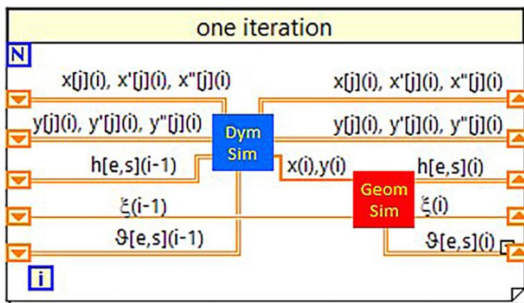
Figure 8. Data flow between dynamic and geometric simulator in each iteration
