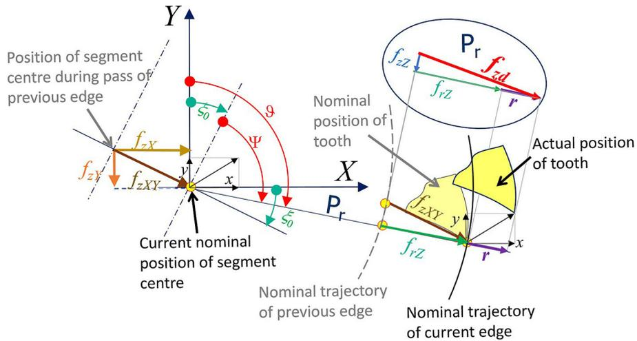
Figure 6. Determination of dynamic feed per tooth
