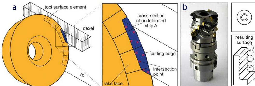
**Figure 3.** Tool and workpiece discretization [12, 13]
