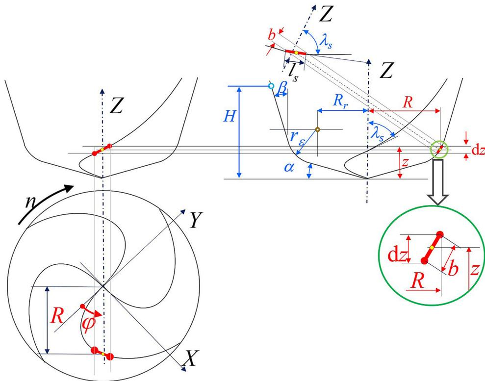
Figure 4. Discretization of universal cutter geometry into segments
