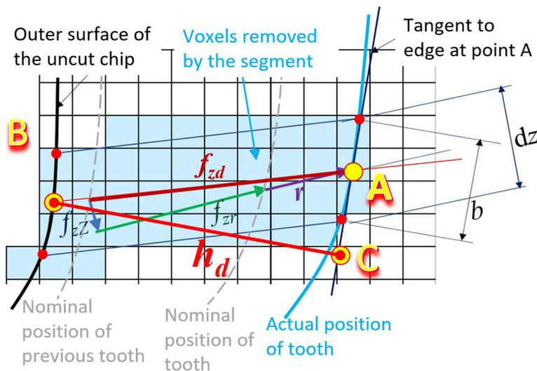
Figure 7. Determination of actual undeformed chip thickness  $h_d$
