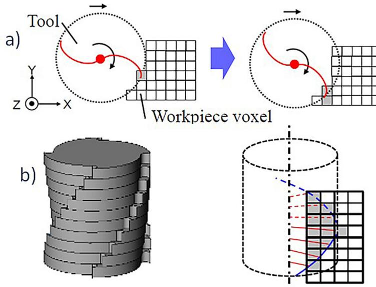
**Figure 2.** Extraction of removal voxels at fine tool rotation angle intervals
