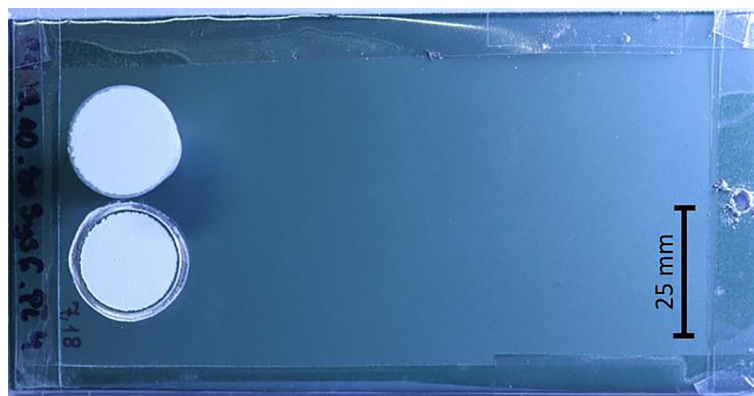
Fig. 6. Example view of sample and dolly after pull-off adhesion test
