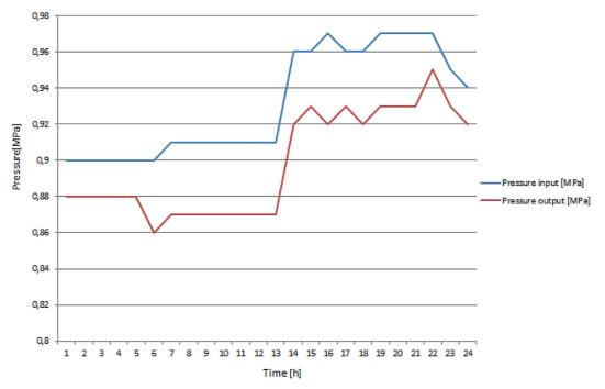
Fig. 6. Difference between input and output pressure in the preliminary heat exchanger nr 2
