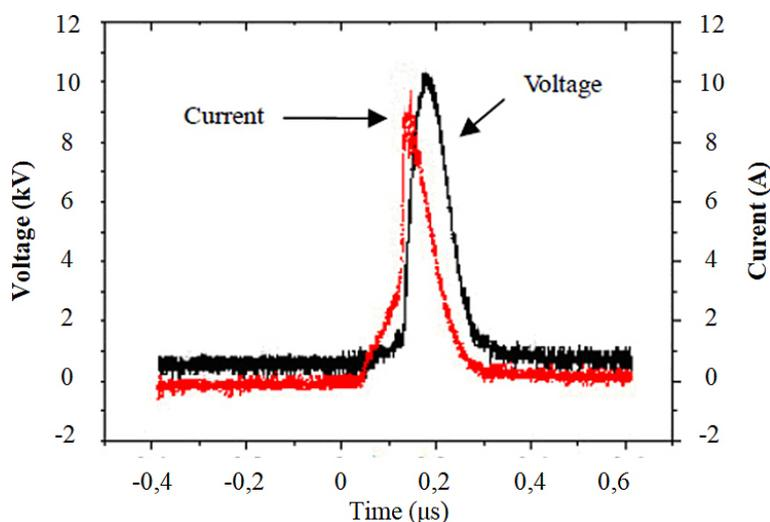
Fig. 3. The waveforms of the applied voltage to and the discharge current during discharge
