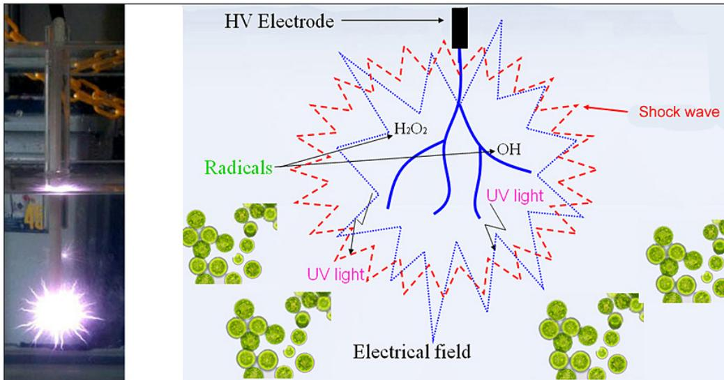
Fig. 4. The discharge phenomena in the water
