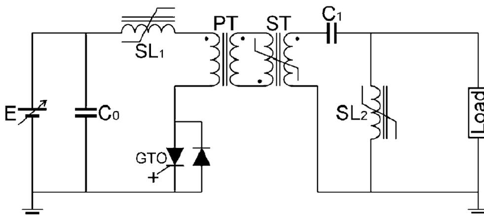
Fig. 1. A diagram of the circuit of the pulse discharge
