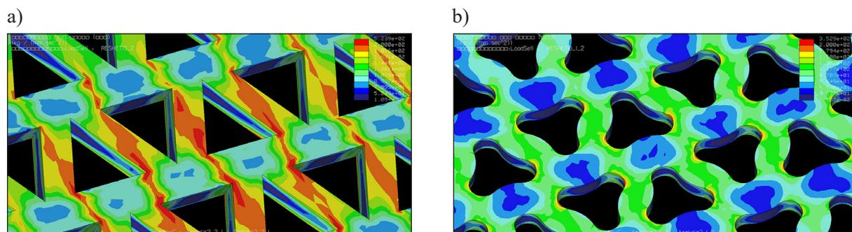
Fig. 6. The nature of the stresses in the central zones of sieves: a – basic sieves with triangular holes; b – developed sieves with activators
