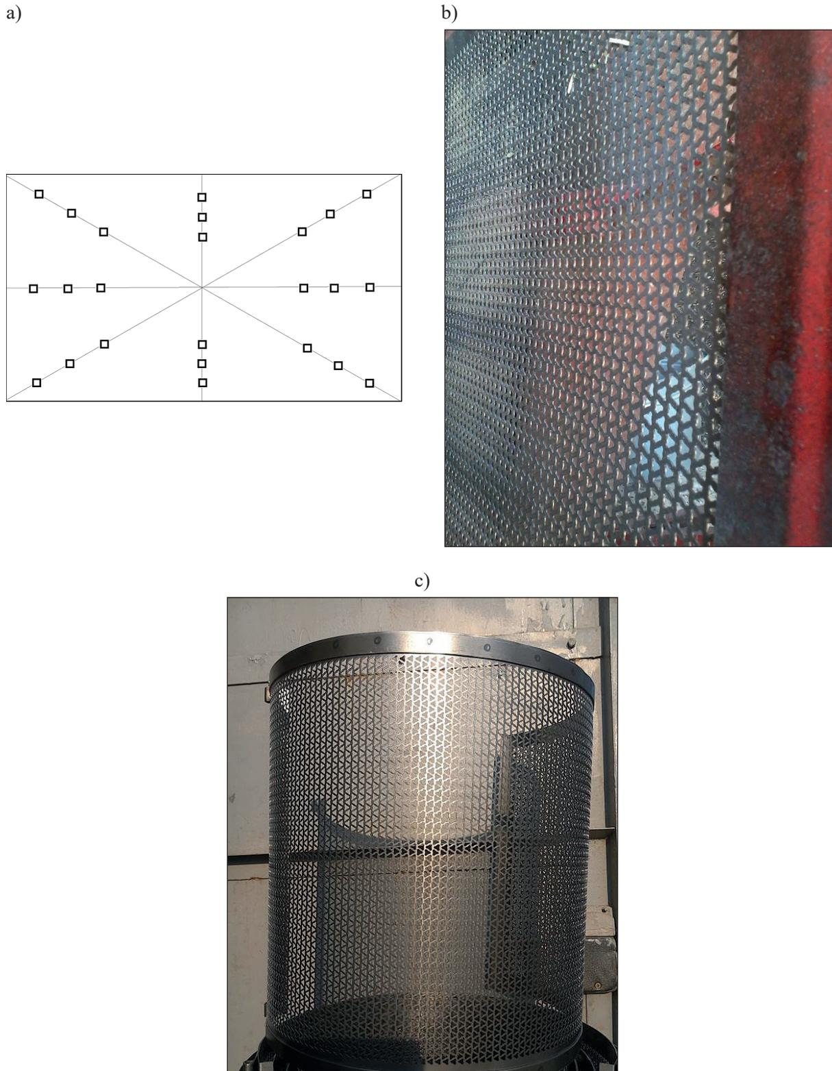
**Fig. 4.** Experimental determination of average thickness of sieves: (a) the scheme of measurements, (b, c) fragments of flat and cylindrical sieves with epicycloid activators (2000 hours of an operating time)
