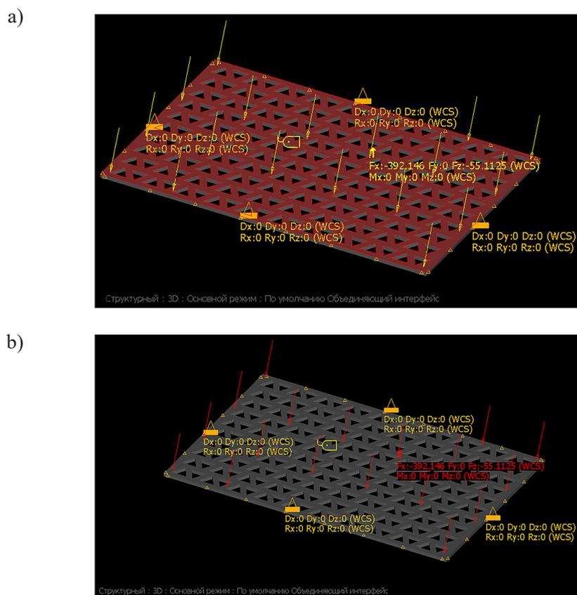
Fig. 3. Fragments of sieve fixing scheme (a) and its loading (b)
