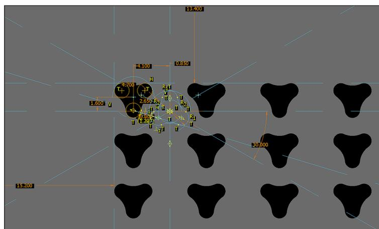
Fig. 2. Fragment of the developed vibrating sieve model with a three-fold epicycloid form of holes
