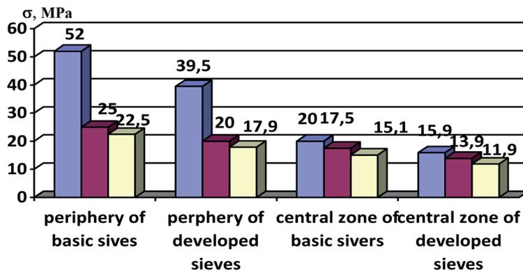
**Fig. 8.** Distribution of equivalent tension on the sections of basic and developed vibrosieves
