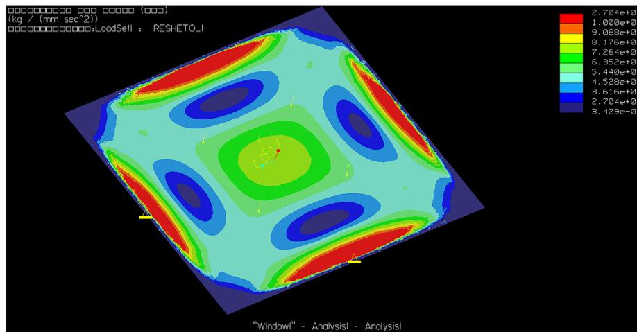
Fig. 5. Character of stress on a vibrating sieve surface: 1 – peripheral zones, 2 – central zones
