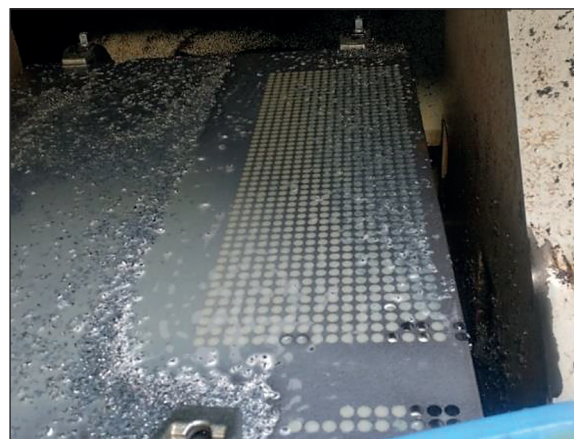
Fig. 1. Cast iron plate with machined holes
