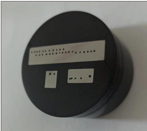
Figure 2. Prepared sample to measure the recast layer
