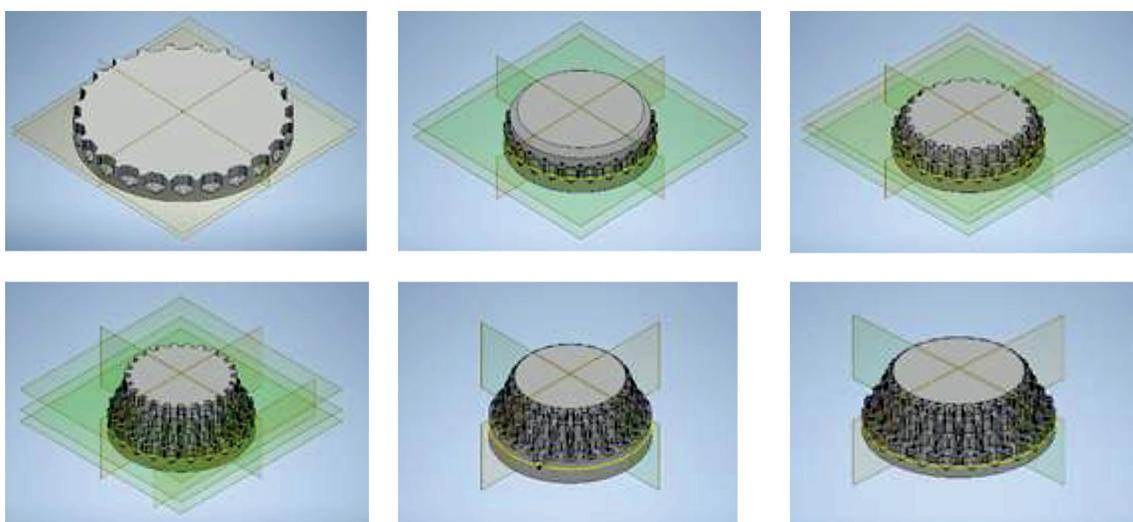
Fig. 4. Stages of 3D modelling the head of the minaret
