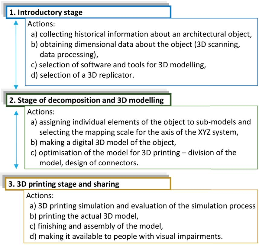
Fig. 1. Procedure for creating digital 3D models dedicated to 3D printing
