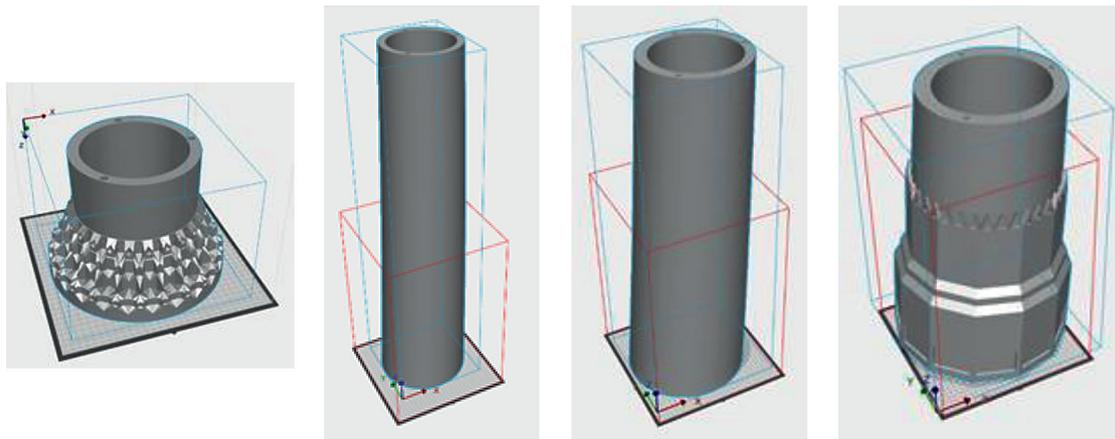
Fig. 5. View of the individual digital elements of the 3D model of the minaret in the Slicer program
