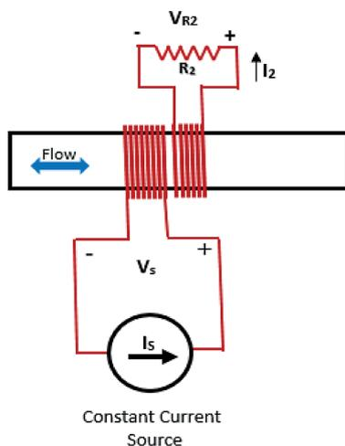
Figure 3. The double coil sensor: Flow rate measurement and direction detection
