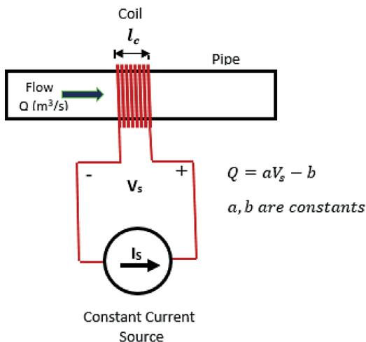
**Figure 1.** The single coil sensor
