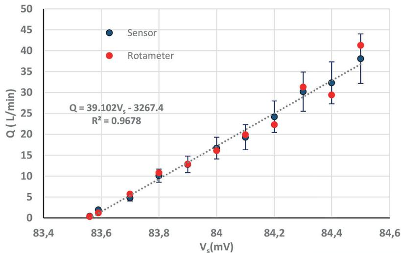
Figure 5. Comparison of the sensor measurements and the rotameter readings
