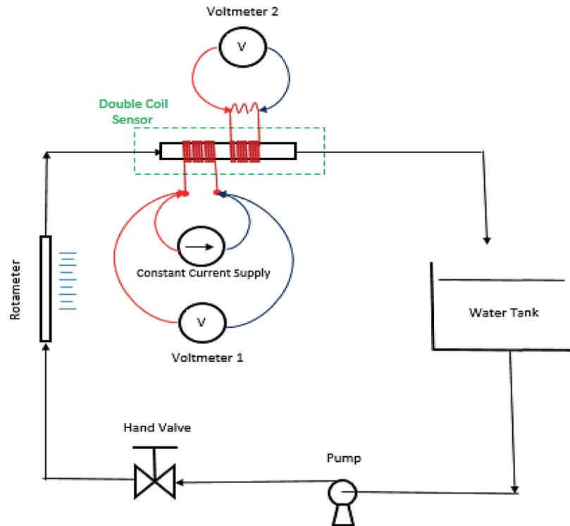
Figure 4. Schematic representation of the equipment used to test the sensor
