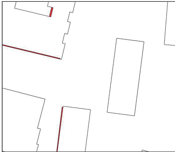
Fig. 9. Consistency of the contour lines of buildings on the master map with their equivalents in CityGML format downloaded from the resources of GUGiK (red colour marks displacement)
