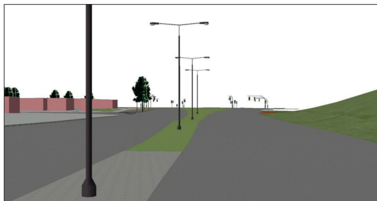
Fig. 10. The result of proposed extension of data with the shape and angle of rotation of light posts and traffic lights
