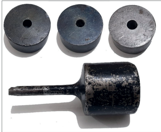
Figure 4. Wire drawing dies and die casing
