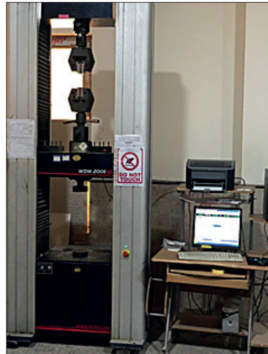
Figure 5. A computerized universal testing machine WDW-200E.
