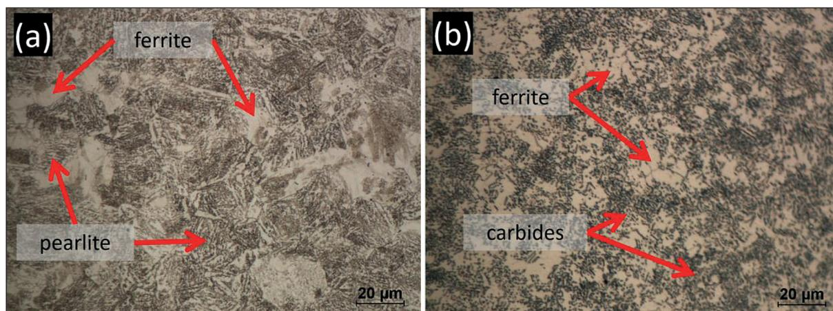
Fig. 8. Effect of annealing on the microstructure of the 42CrMo4 steel. As-received (a) and (b) annealed steel, LOM
