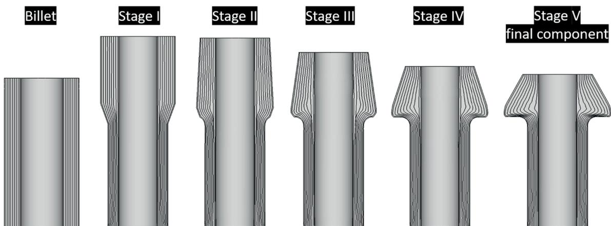
Fig. 6. Simulation of flow lines arrangement at different stages of forming, FEM
