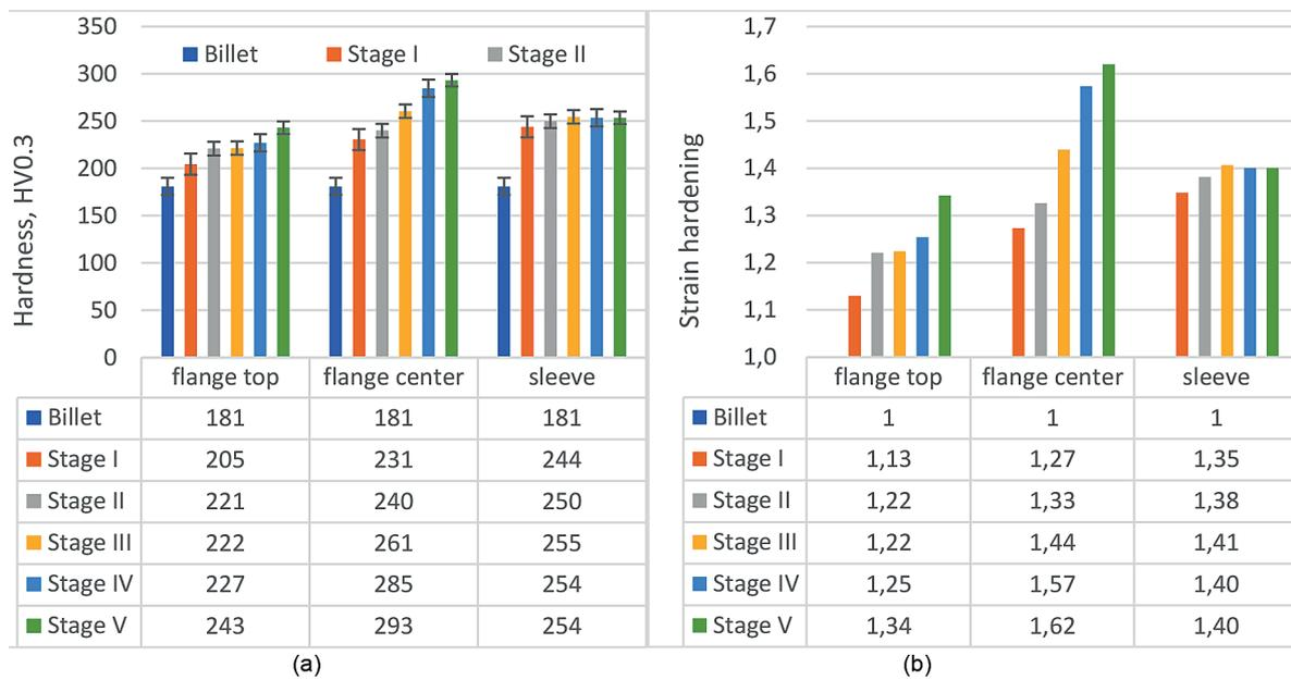
**Fig. 11.** Hardness results of specific areas of cold-formed hollow parts: (a) Vickers hardness; (b) strain hardening at different stages of metal forming
