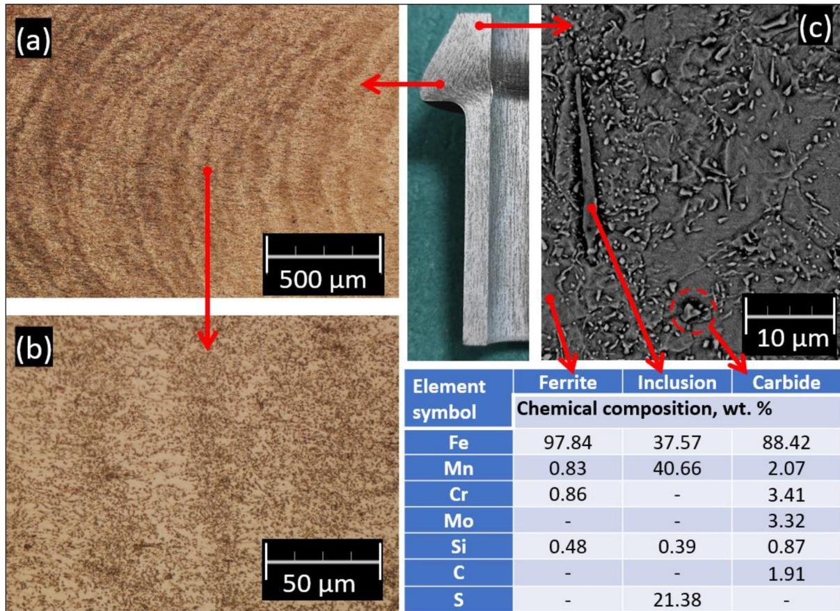
Fig. 9. Macro- and microstructure in different areas of plastic deformation (a, b) LOM; (c) microstructure and results of spot chemical analysis, SEM-EDS
