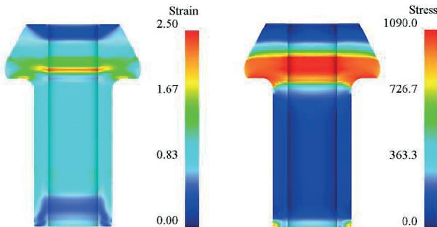
Fig. 4. The forging's highest strain and stress areas at the final stage of cold-forming, following the results of comparable forming technology [36], FEM
