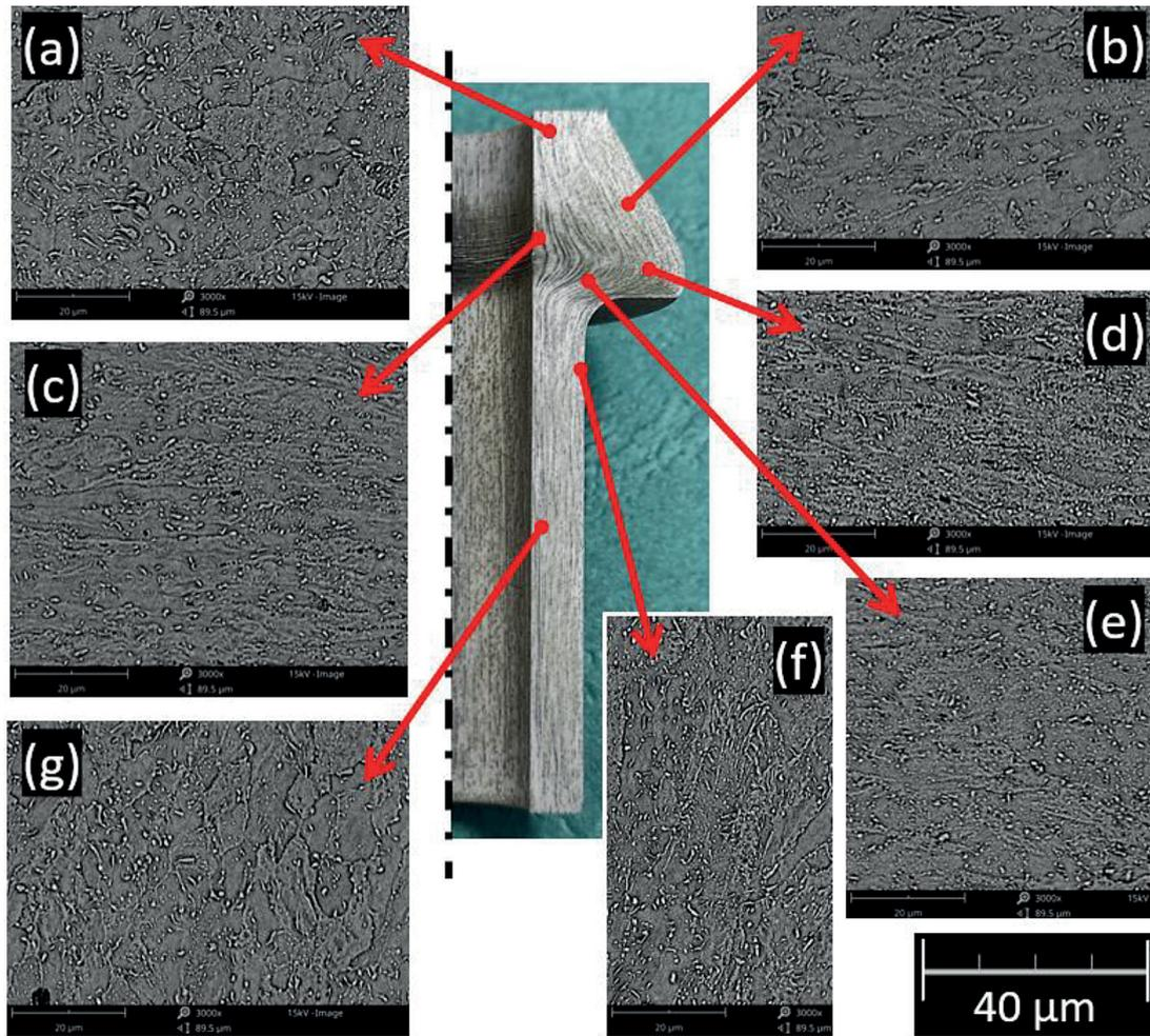
**Fig. 10.** Microstructure and grain arrangement in different locations of final component cross-section: flange top (a, b); flange center (c-e); sleeve (g, h), SEM
