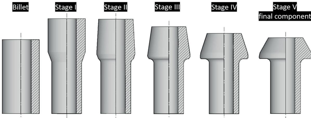
Fig. 2. Idea of the five stages forming process: I stage – extrusion, II-V stages – flange upsetting
