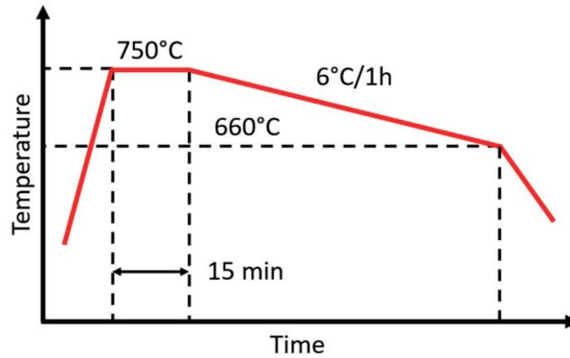
Fig. 3. Annealing process parameters utilized for 42CrMo4 sleeve batch
