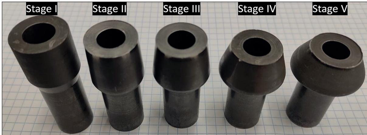
Fig. 5. Fabricated forgings at five stages of forming
