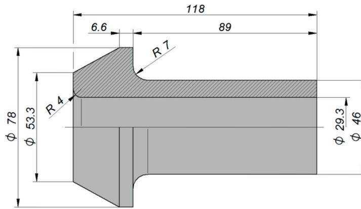
Fig. 1. Dimensions of the 42CrMo4 steel hollow component with the outer flange [35]
