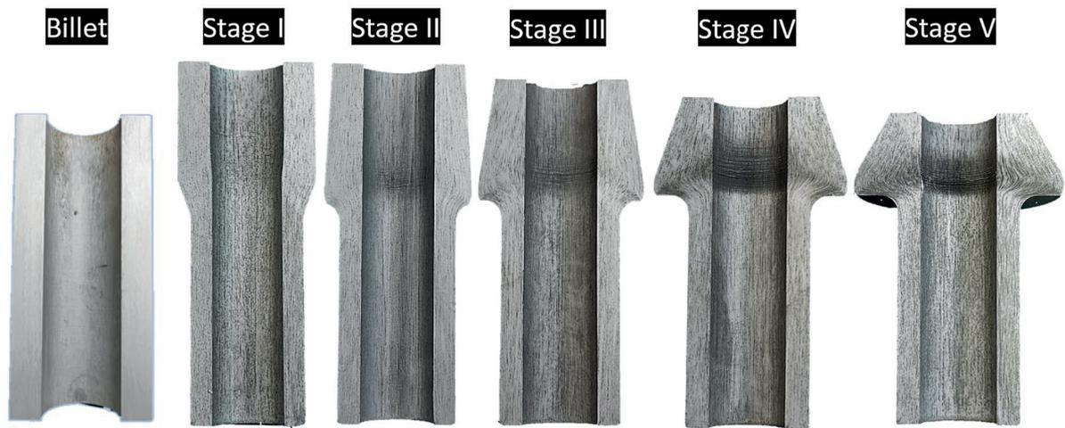
Fig. 7. Macrostructure of a hollow flanged component at different stages of forming, macroetching
