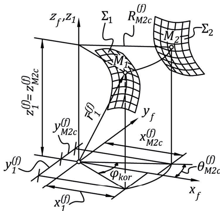
Figure 4. Tooth flanks in the  $n^{\text{th}}$  position
