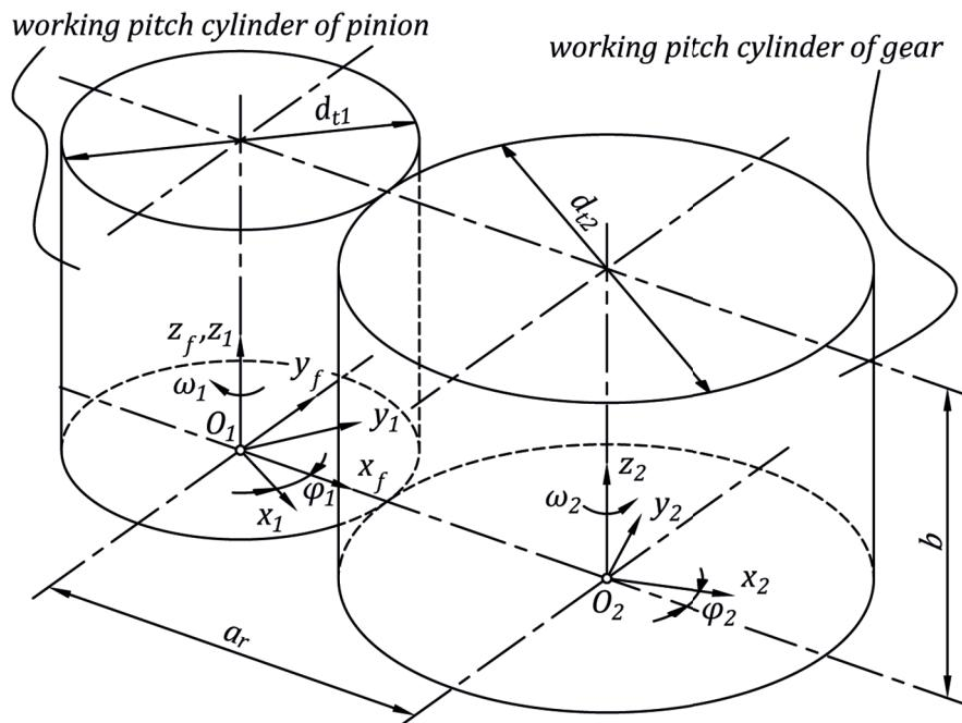
**Figure 1.** Coordinate systems set up in the cylindrical gear pair mesh analysis
