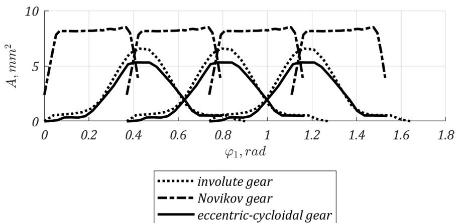
**Figure 10.** Contact areas as a function of pinion rotation angle.
