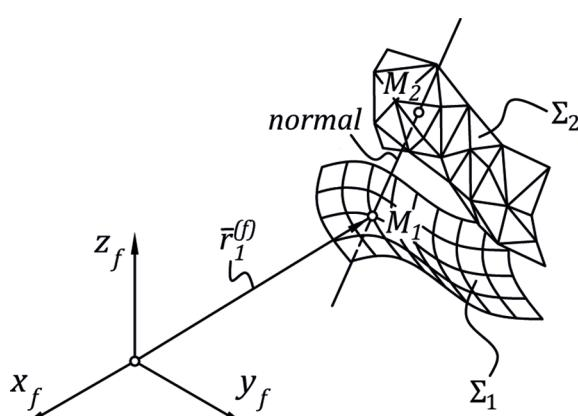
**Figure 6.** The proposed method for determining distances between mating tooth surfaces
