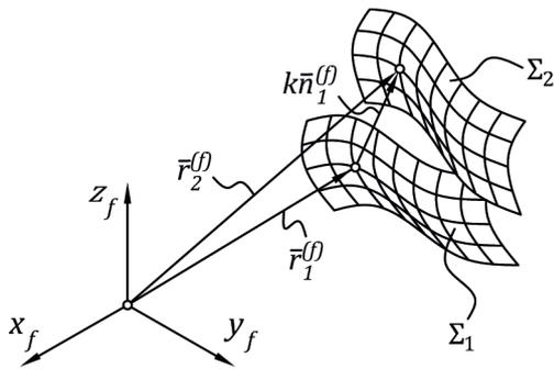
**Figure 5.** Determining distances between mating tooth surfaces
