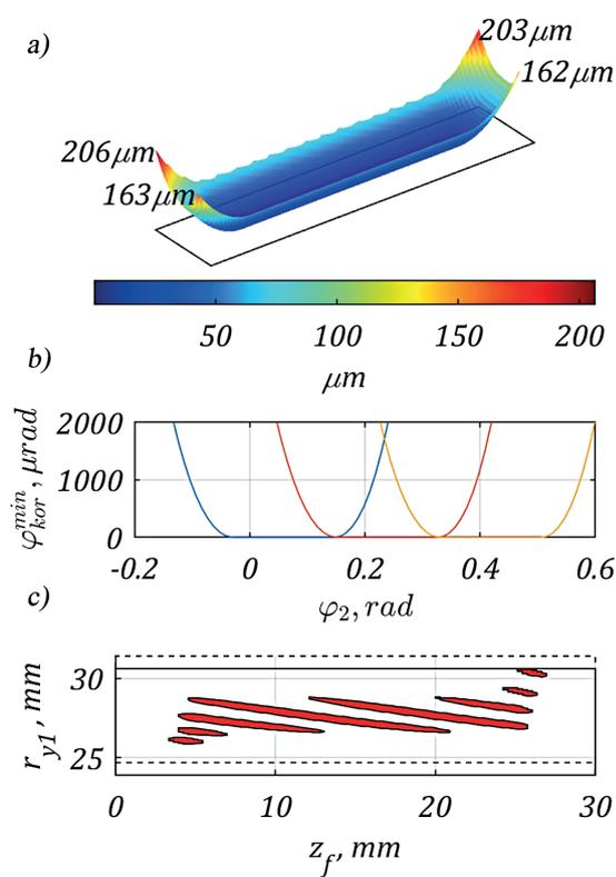
**Figure 7.** Results of tooth contact analysis for the involute gear pair: a) Ease-Off topography, b) transmission chart, c) contact patterns.
