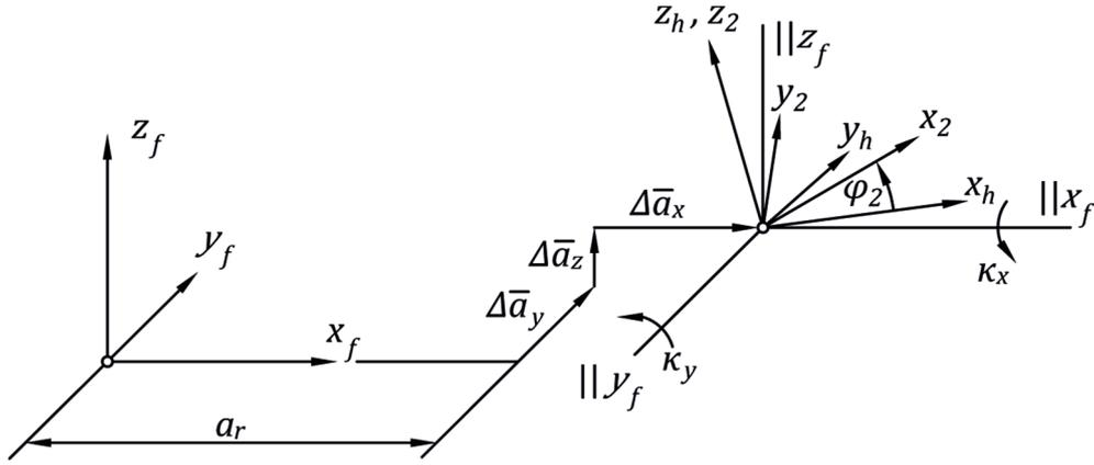
Figure 2. The position and orientation of additional coordinate system h
