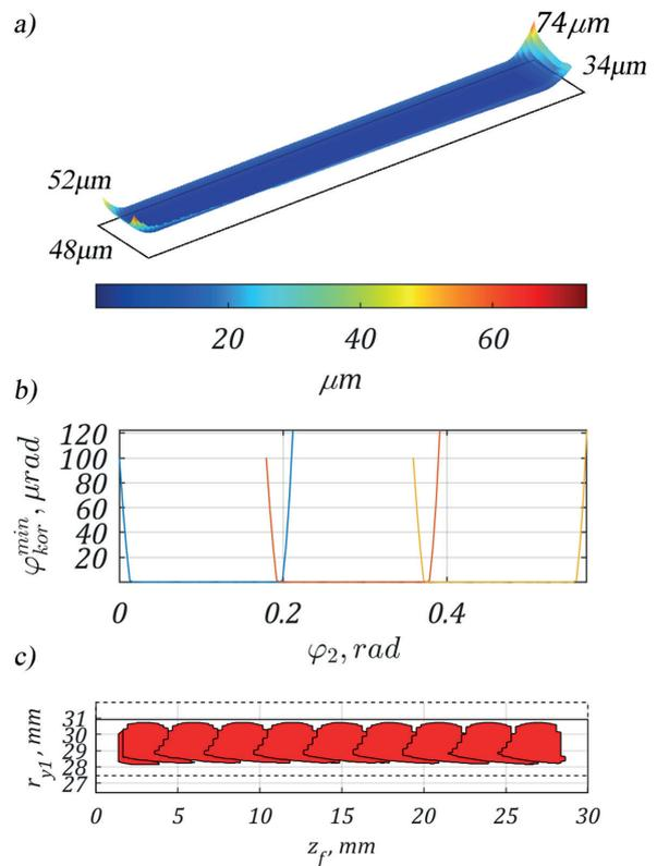
**Figure 8.** Results of tooth contact analysis for the Novikov gear pair: a) Ease-Off topography, b) transmission chart, c) contact patterns
