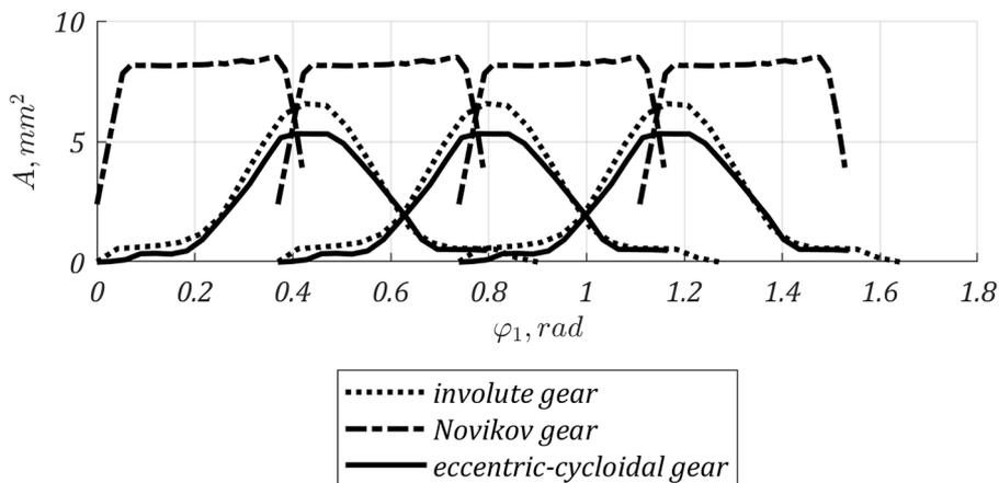
**Figure 10.** Contact areas as a function of pinion rotation angle.
