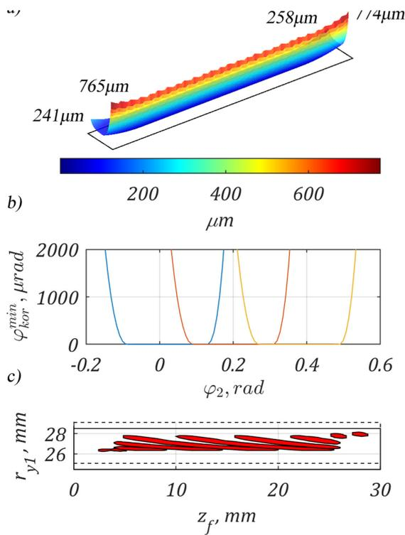
**Figure 9.** Results of tooth contact analysis for the eccentric-cycloidal gear pair: a) Ease-Off topography, b) transmission chart, c) contact patterns
