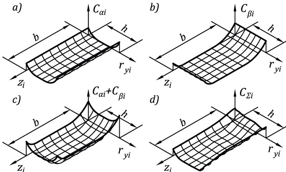
Figure 3. Types of tooth flank modifications: a) profile modification, b) flank line modification, c) simultaneous profile and flank line modification, d) topological modification, where b is the toothed ring width, and h is the tooth height
