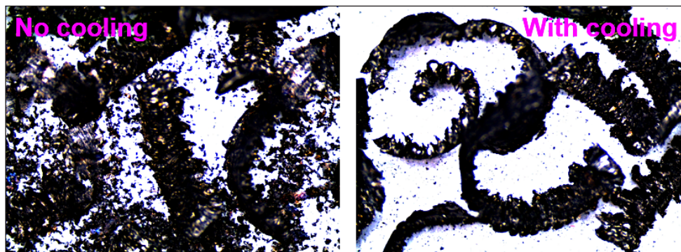
Fig. 10. Comparison of the morphology of chips obtained for cutting: a) without cooling, b) with cooling of the cutting tool. Magnification 9.5 x
