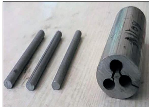
**Fig. 2.** Wear testing specimens
