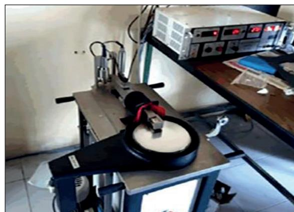
**Fig. 3.** Pin-on-disc testing apparatus
