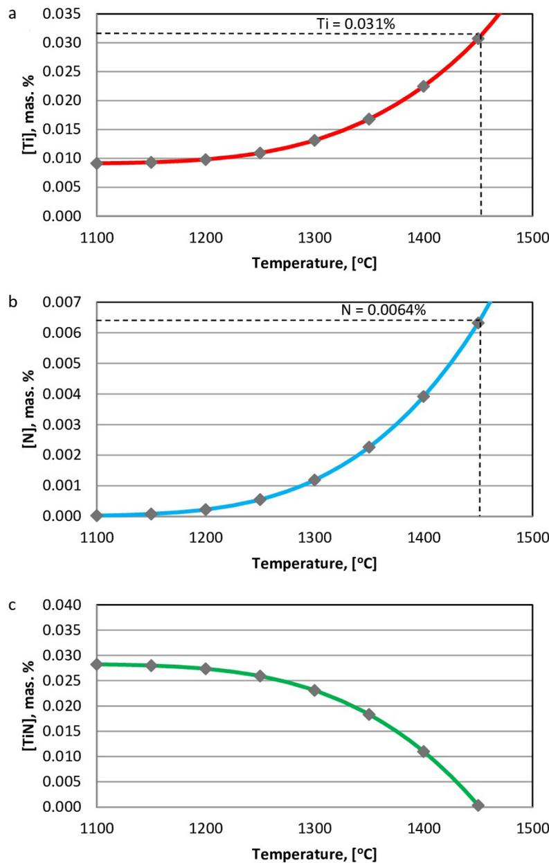
**Fig. 1.** The results of calculations of the precipitation of the TiN interstitial phase in the austenite of the tested steel containing 0.031% Ti and 0.0064% N: a) change in the concentration of Ti dissolved in austenite depending on the temperature, b) change in the concentration of N dissolved in austenite depending on the temperature, c) change in the proportion of TiN phase undissolved in austenite depending on the temperature
