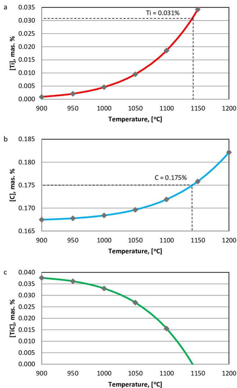
**Fig. 2.** The results of calculations of the precipitation of the TiC interstitial phase in the austenite of the tested steel containing 0.031% Ti and 0.175% C: a) change in the concentration of Ti dissolved in austenite depending on the temperature, b) change in the concentration of C dissolved in austenite depending on the temperature, c) change in the proportion of TiC phase undissolved in austenite depending on the temperature
