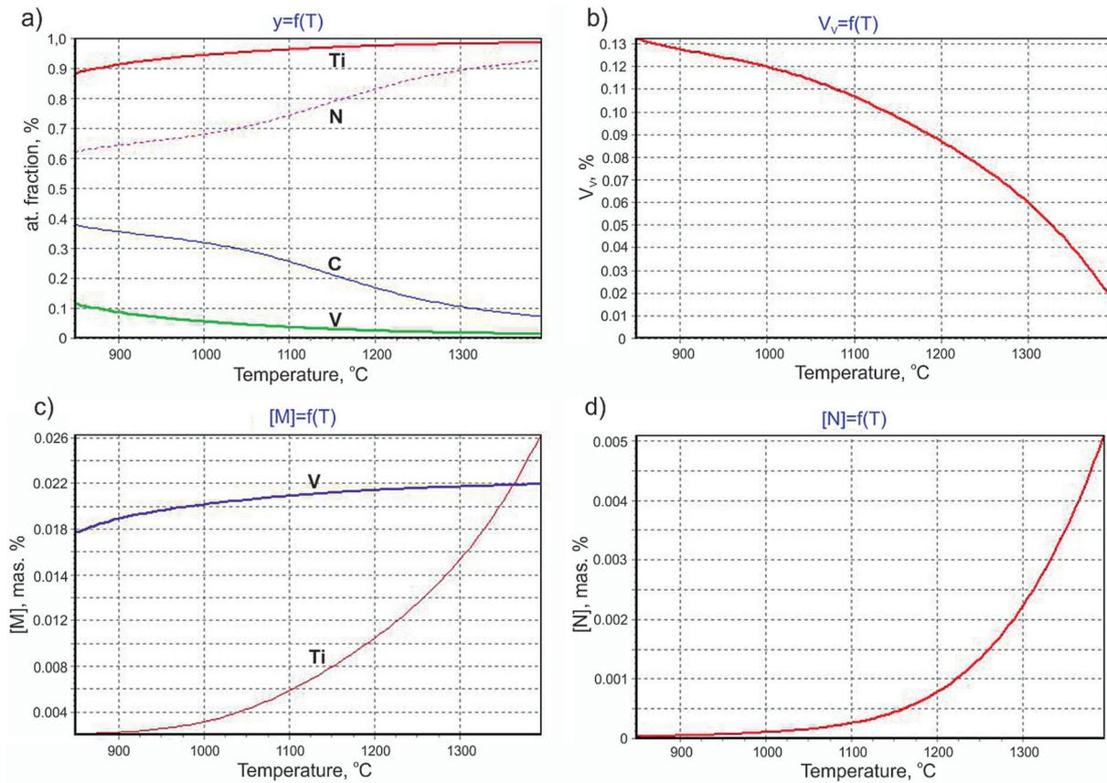
**Fig. 5.** The results of the analysis of thermodynamic equilibrium conditions: a) chemical composition of the complex carbonitride, b) volume fraction,  $V_v = f(T)$ , c) fractions of titanium and vanadium,  $[M] = f(T)$ , d) fraction of nitrogen  $[N] = f(T)$
