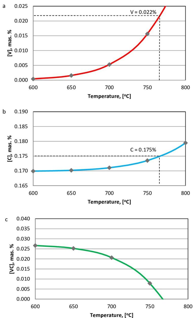
**Fig. 4.** The results of calculations of the precipitation of the VC interstitial phase in the austenite of the tested steel containing 0.022% V and 0.175% C: a) change in the concentration of V dissolved in austenite depending on the temperature, b) change in the concentration of C dissolved in austenite depending on the temperature, c) change in the proportion of VC phase undissolved in austenite depending on the temperature
