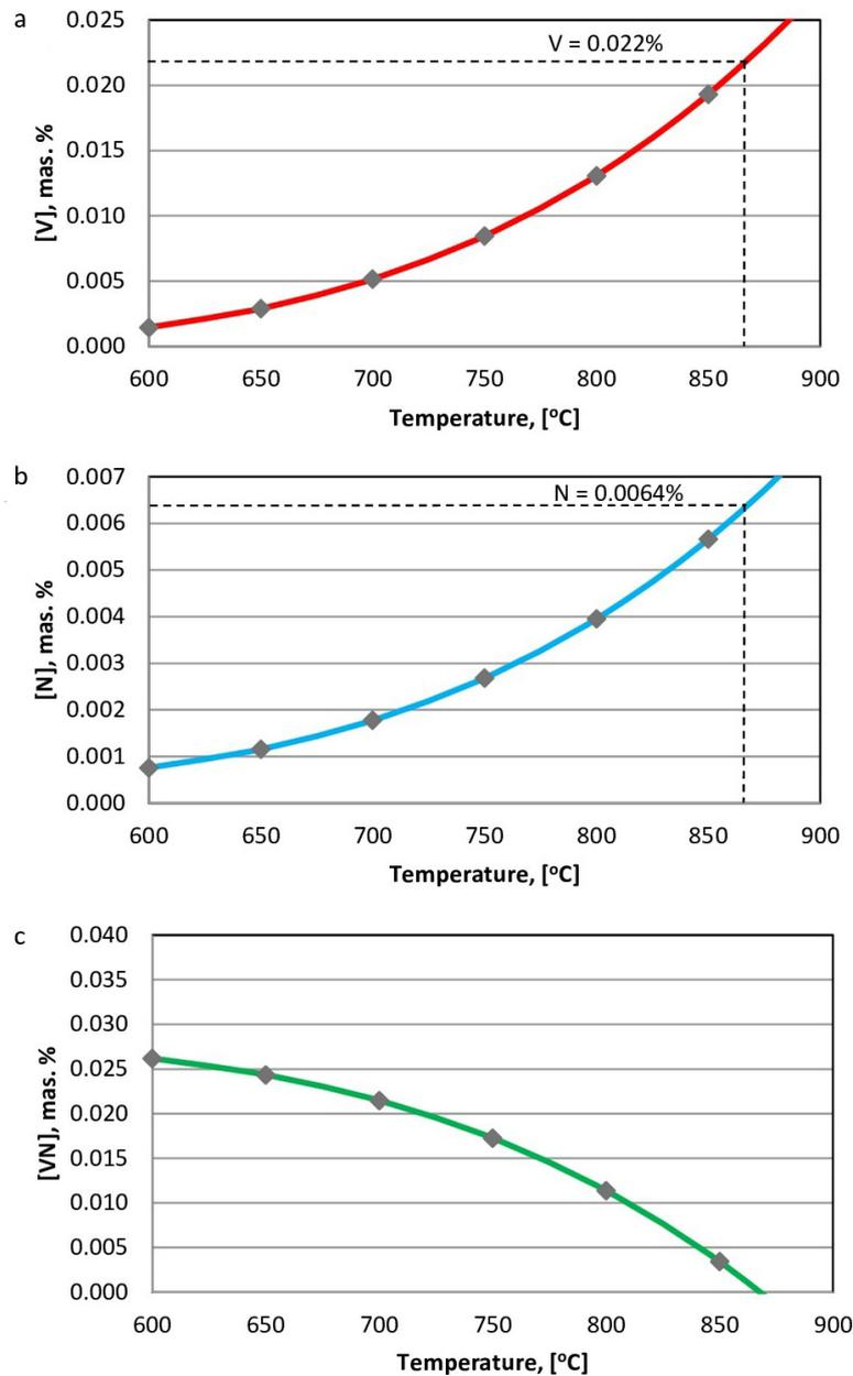
**Fig. 3.** The results of calculations of the precipitation of the VN interstitial phase in the austenite of the tested steel containing 0.022% V and 0.0064% N: a) change in the concentration of V dissolved in austenite depending on the temperature, b) change in the concentration of N dissolved in austenite depending on the temperature, c) change in the proportion of VN phase undissolved in austenite depending on the temperature
