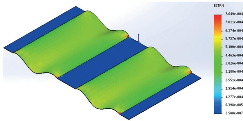
Fig. 7. Strain of the load-bearing floor under loading
