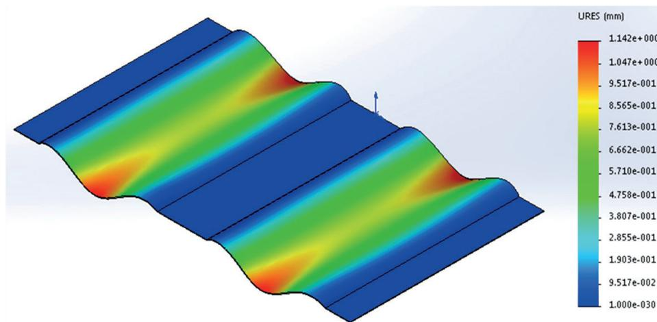
Fig. 6. Displacement of the load-bearing floor under loading
