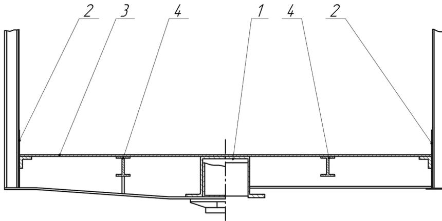
**Fig. 2.** Sketch of the cross-section of SBRFC (cross-section of the beam and pivot in the middle of the frame): 1 – spinal beam; 2 – lower trim of the side wall; 3 – load-bearing floor; 4 – cross-beam
