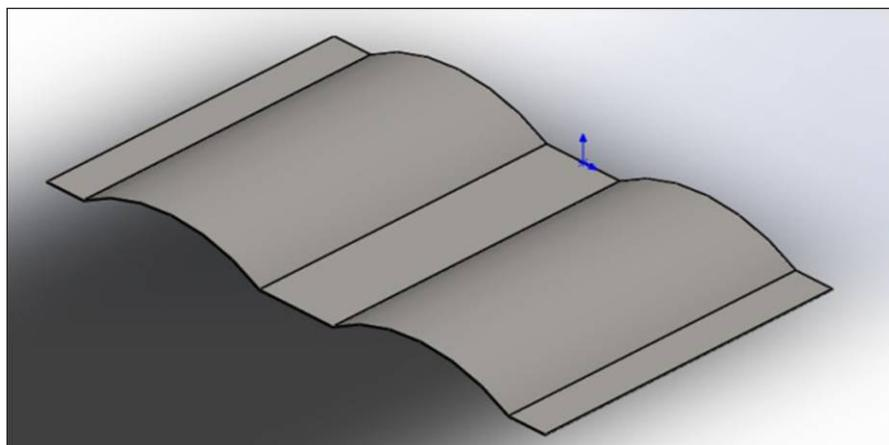
**Fig. 3.** Profile of the SBRFC load-bearing floor
