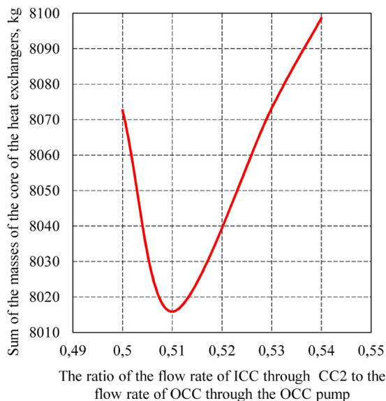
**Fig. 8.** Dependence of  $M_{\Sigma}$  on the ratio  $G_{ww2}/G_{ww}$  (outboard water flow through central cooler 2 to sea water flow through the pump); at:  $t_{w1} = 39.7\text{ }^{\circ}\text{C}$ ;  $t_{w11} = 38\text{ }^{\circ}\text{C}$ ;  $t_{w12} = 55.2\text{ }^{\circ}\text{C}$ ,  $G_{ww1}/G_{ww} = 0.37$
