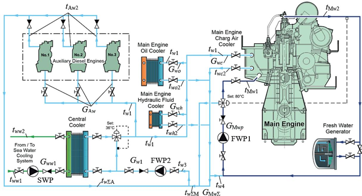
Fig. 1. Scheme of the cooling system of a ship power plant with one central cooler: FWP – fresh water pump; SWP – sea water pump
