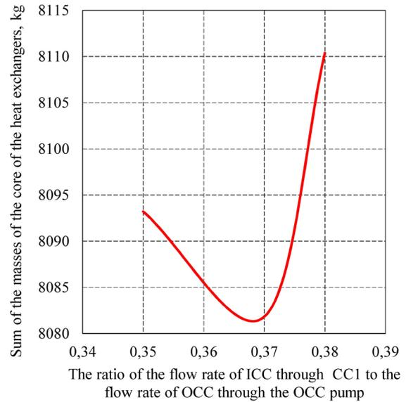
**Fig. 7.** Dependence of  $M_{\Sigma}$  on the ratio  $G_{ww1}/G_{ww}$  (outboard water flow through central cooler 1 to sea water flow through the pump); at:  $t_{w1} = 39.7\text{ }^{\circ}\text{C}$ ;  $t_{w11} = 38\text{ }^{\circ}\text{C}$ ;  $t_{w12} = 55.2\text{ }^{\circ}\text{C}$ ,  $G_{ww2}/G_{ww} = 0.52$
