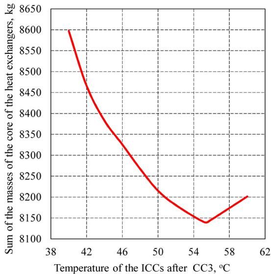
**Fig. 6.** Dependence of  $M_{\Sigma}$  on the temperature of the ICC after central cooler 3,  $t_{w12}$ , at  $t_{w1} = 39.7\text{ }^{\circ}\text{C}$ ;  $t_{w12} = 37.3\text{ }^{\circ}\text{C}$ ,  $G_{ww1}/G_{ww} = 0.34$ ;  $G_{ww2}/G_{ww} = 0.52$
