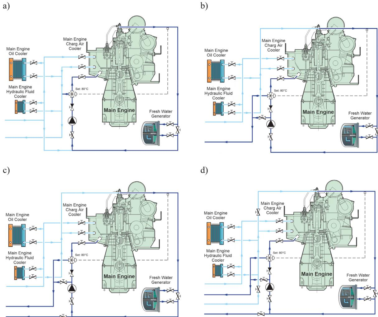
Fig. 2. Alternative schemes of the cooling system with one central cooler
