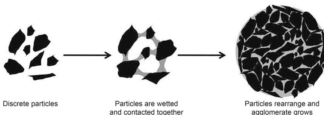
Fig. 1. The process of agglomeration mechanism with organic binder [1]
