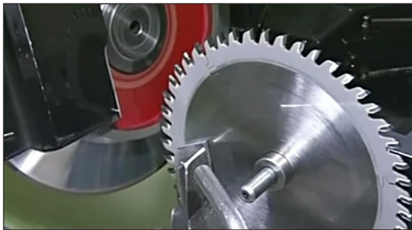
Fig. 8. External grinding of saw blade teeth
