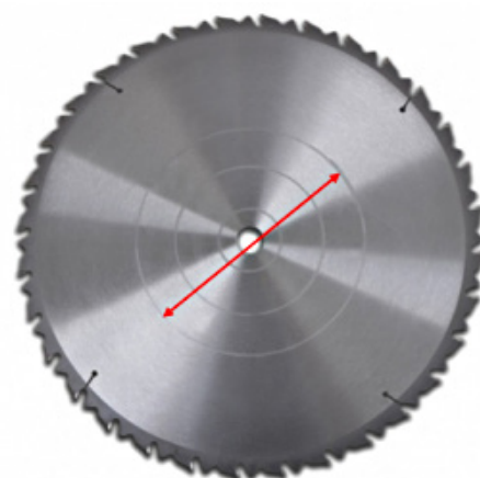
Fig. 15. Measuring the saw blade diameter
