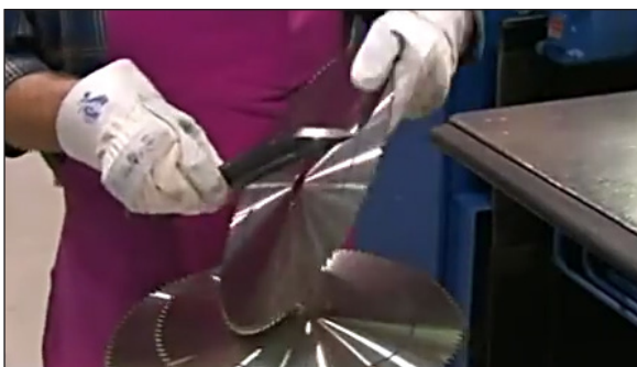
Fig. 4. Manual measurement of disc grooves unevenness
