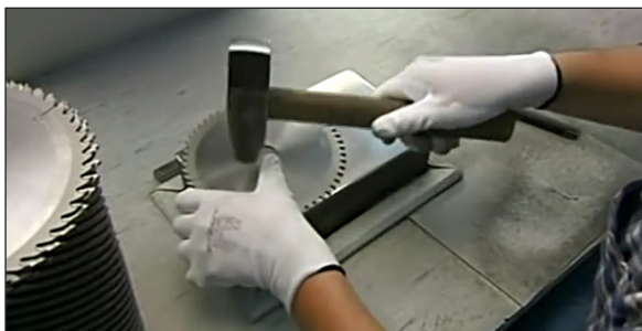
Fig. 9. Manual knocking of saw blade unevenness
