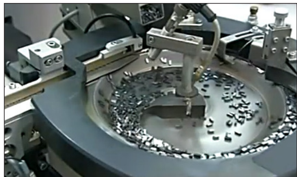
Fig. 6. Carbide tips check laser control
