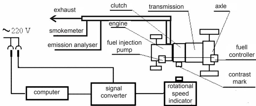
Fig. 2. General scheme of the testing equipment
