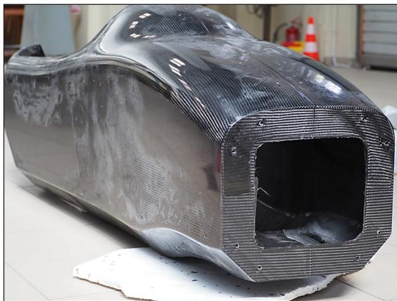
**Figure 9.** Final product after extraction from the molds
