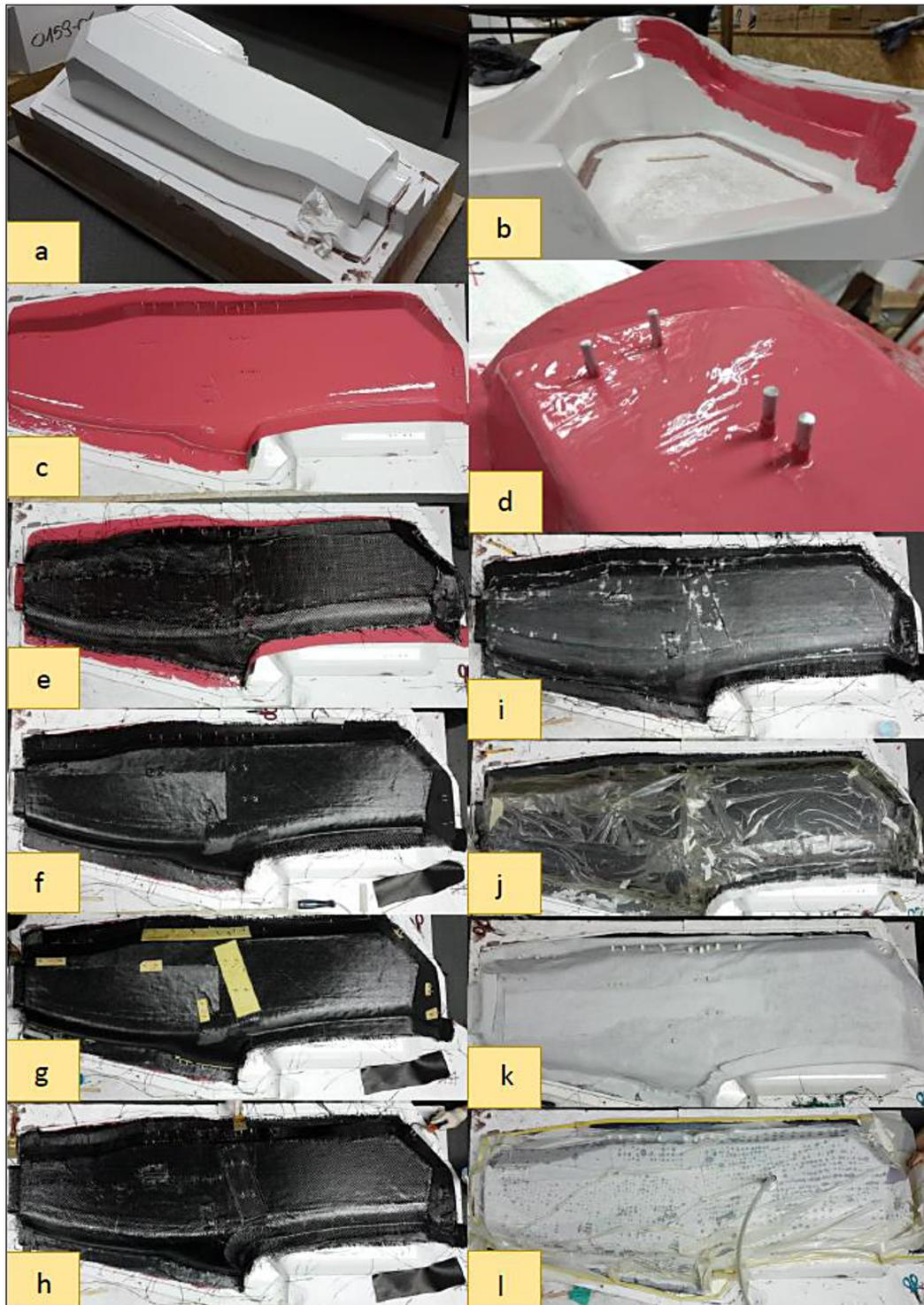
Figure 4. Mold manufacturing process
